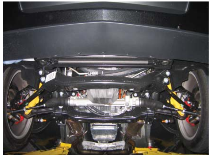
Underside Body Cladding Removed
