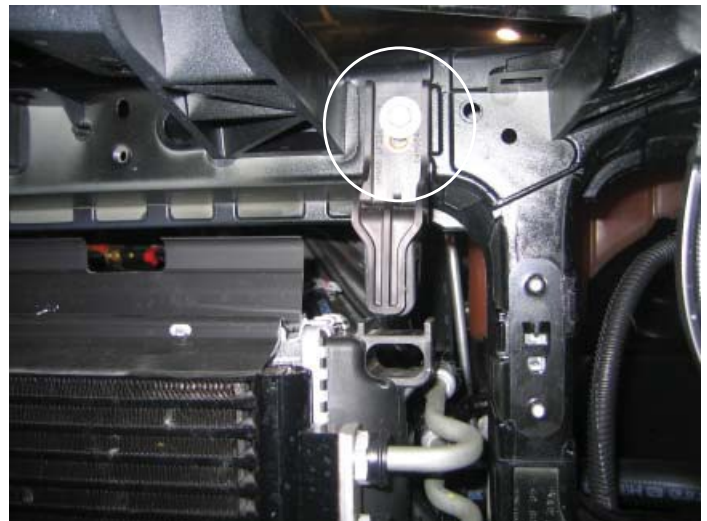
Radiator Upper Mount Bolts (Driver's Side)
