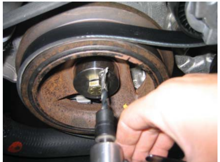
Drilling the Crank
