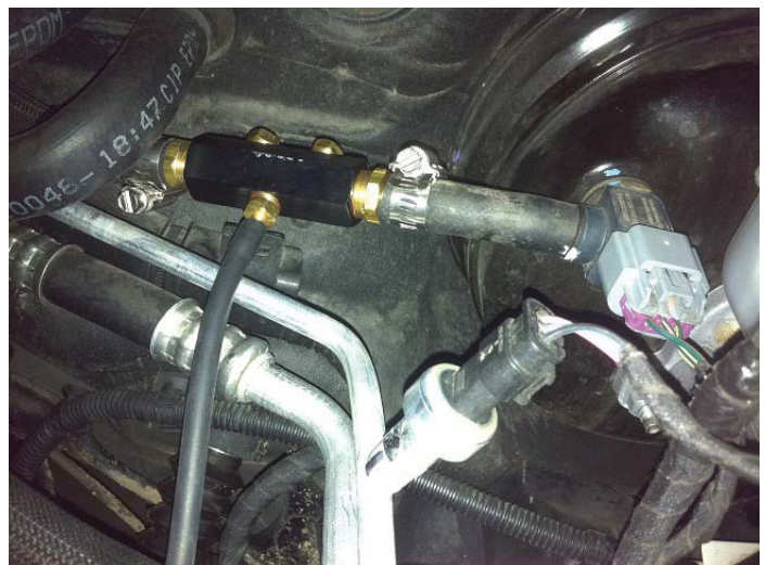
Vacuum Manifold Installed
