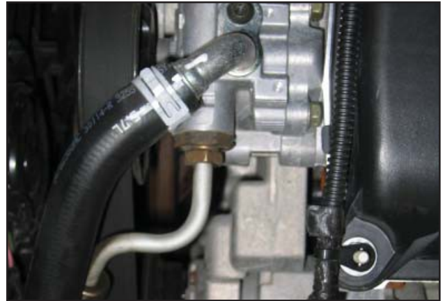
Power Steering Hose's Original Position
