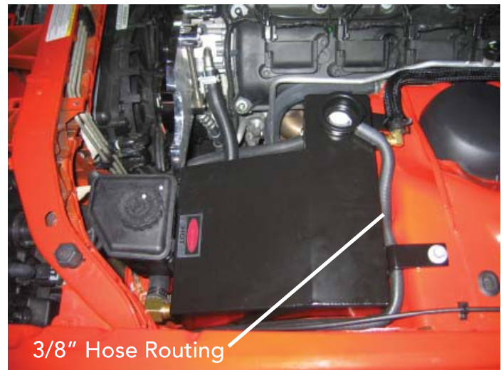
Coolant Hose Routing
