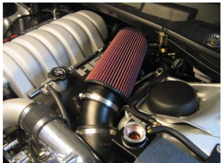
Air Inlet Installed
