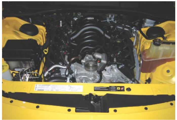
Engine Air Filter Removed
