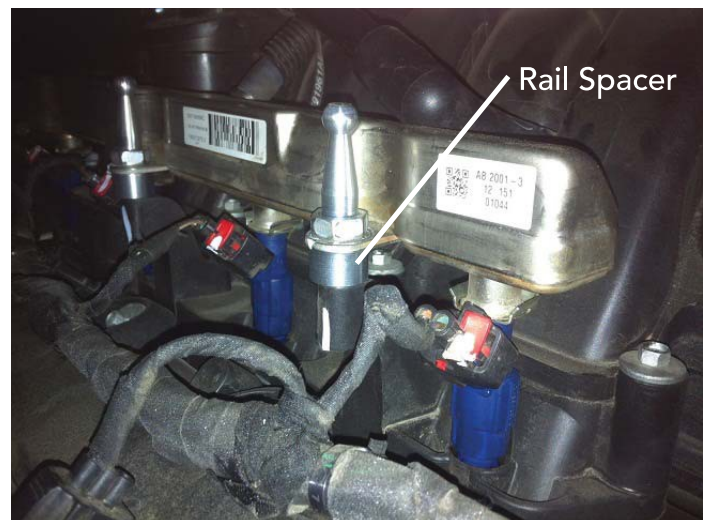
Fuel Rails Installed
