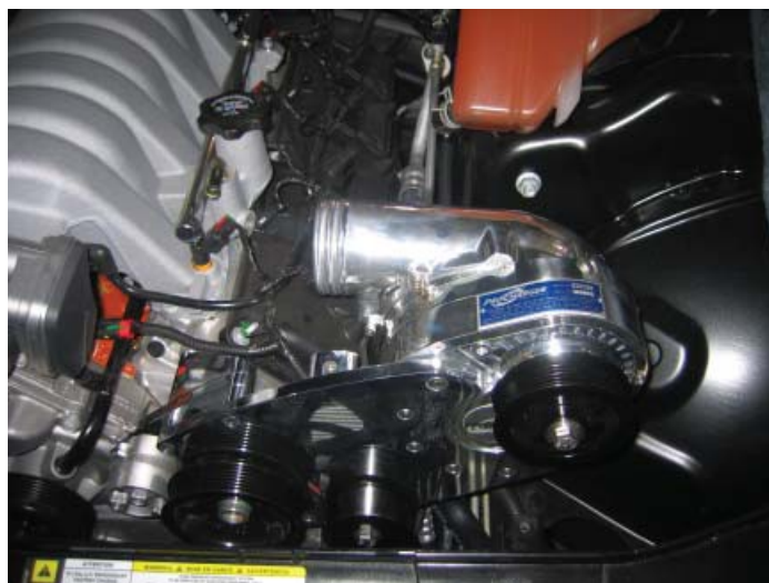
ProCharger Head Unit Installed
