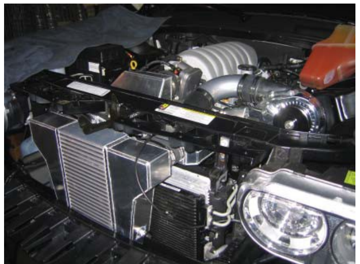
Intercooler and Tubing Installed
