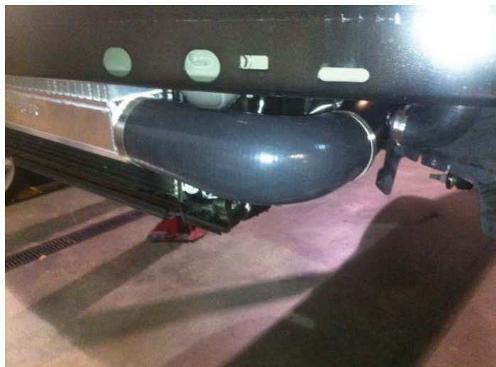
Lower Intecooler Tubing Installed
