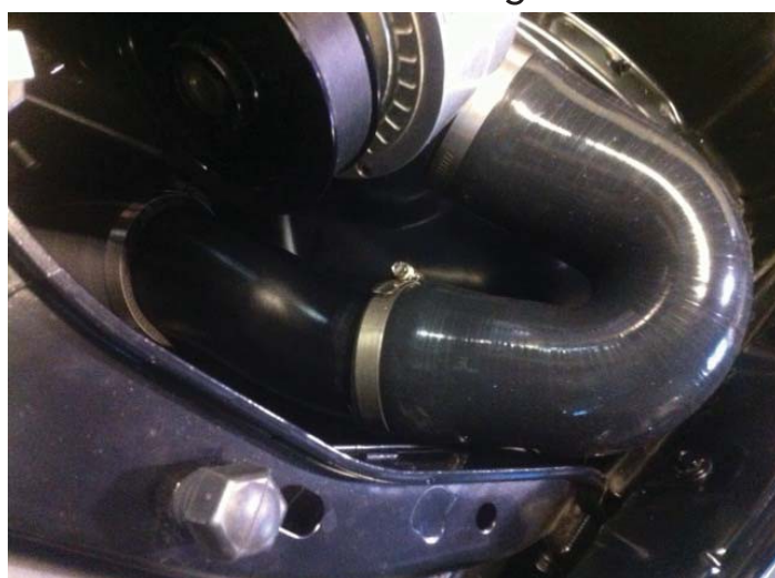
Silicone 135° Elbow Installed
