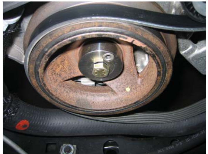
Drill Jig Installed
