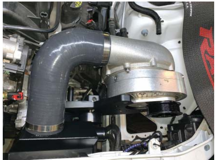
Tube and Reducer Installation
