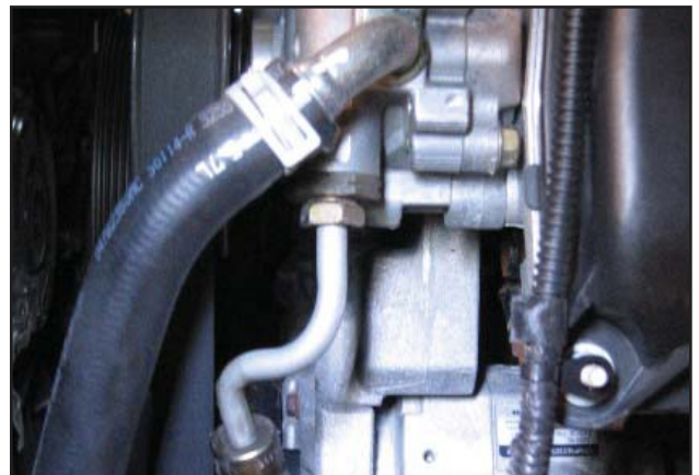
Power Steering Hose's New Position
