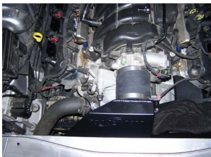
Airbox Tubing Installed
