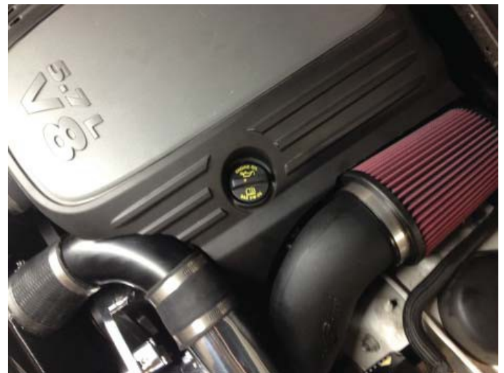
Air Inlet Installed
