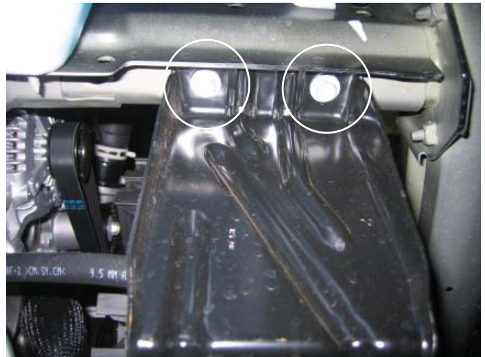
Radiator Cradle Bolts (Pass. Side)
