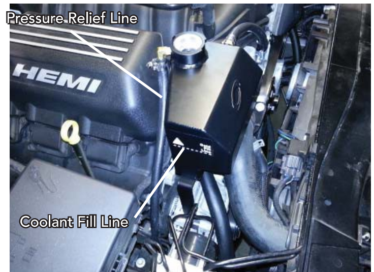
Pressure Relief Line Routing &amp; Fill Line
