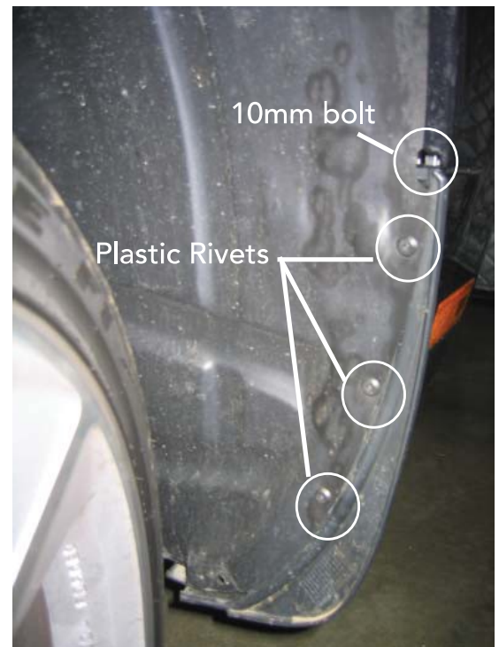
Fascia Connections (Pass. Side)
