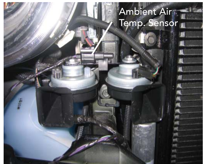
Horn Relocation H.O.
