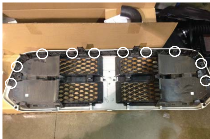
Prepare to Remove Air Deflectors (if equipped) by Removing the Upper Grill
