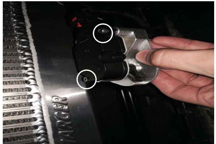
Remove Shutter Motor Cover and Screws
