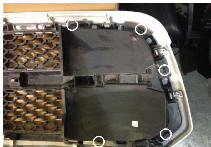
Unclip & Remove Both Grill Air Deflectors
