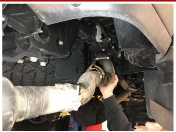
Carefully remove the passenger side tailpipe from the vehicle.
