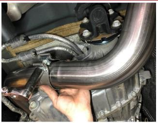
3. Locate the CORSA connector pipe and a 3.0" clamp. Position the 3.0" clamp onto the inlet of the connector pipe with the clamp hardware on the rear side of the pipe and the clamp nut facing down. Insert the connector pipe inlet onto the driver side head pipe outlet as shown, making sure to have at least 1.75" of overlap at the slip fit connection, then snug the clamp using a 15mm socket and 3/8" ratchet, leaving it loose enough for later adjustment.
