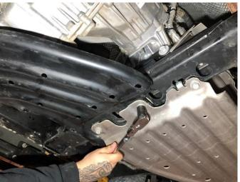
14. Remove the three bolts securing the underside of the skid plate using a 16mm socket and 3/8" ratchet. Slide the skid plate rearward and then move it down to free it from the vehicle. Set aside the skid plate and mounting hardware to be reused during INSTALL STEP 29.
