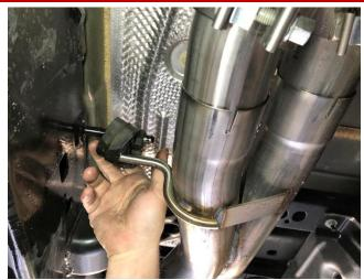
Insert the front muffler/muffler delete hanger into the front exhaust grommet as shown.
