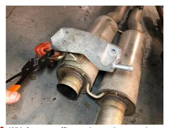
12. With factory muffler section on the ground, use grommet pullers or similar device to remove the rear muffler hanger from the grommet. Note the orientation of the hanger grommet before removal. Set aside the rear muffler hanger mount to be reused during INSTALL STEP 5.
