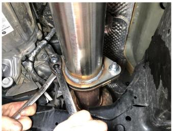
2. Locate the CORSA passenger side head pipe assembly, and the rest of the supplied M10 mounting bolts and nuts for the hardware kit. Install the passenger side head pipe onto the flange from the passenger side catalytic converter as shown and secure the flange with the M10 flange bolts and nuts, using two 15mm wrenches.
