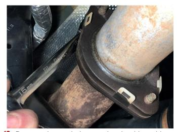
16. Remove the two bolts securing the driver side "Y" pipe flange using a 16mm wrench. The factory bolts securing the flanges will not be reused.
