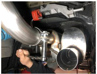
11. Locate the CORSA driver front tailpipe and a 3.0" clamp. Position the 3.0" clamp onto the outlet of the muffler/muffler delete with the clamp hardware facing away from the driveshaft and the clamp nut facing down. Insert the tailpipe inlet into the muffler outlet, making sure to have at least 1.75" of overlap at the slip fit connection, then snug the clamp using a 15mm socket and 3/8" ratchet, leaving it loose enough for later adjustment.
