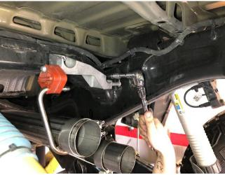
**8.** Locate the two nuts set aside in **REMOVAL STEP 10**. Reinstall the rear muffler hanger mount onto the two studs on the vehicle chassis in the factory location using the retained factory hardware. Tighten the two nuts using a 13mm socket and 3/8" ratchet.
