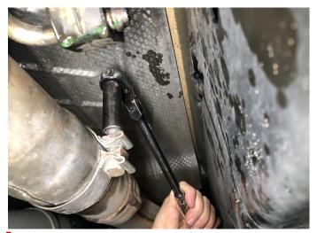
Using a 15mm socket and 3/8" ratchet, loosen the outer factory clamp securing the stock muffler section to the factory "Y" pipe.
