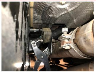
9. Using grommet pullers or similar device, remove the front muffler hanger from the grommet. IMPORTANT NOTE: At this time, support the underside of both the factory "Y" pipe and muffler section using adjustable support stands (or equivalent), as the entire stock exhaust will be free to drop down once the rear muffler hanger mount is unbolted from the chassis in the following step. A second person may be needed to assist with this step.
