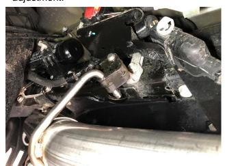
**13.** Locate the CORSA driver rear tailpipe assembly and a 3.0" clamp. Position the 3.0" clamp onto the tailpipe inlet with the clamp hardware on the front side of the pipe, and the clamp nut facing down. Insert the driver rear tailpipe hanger into the exhaust grommet as shown.
