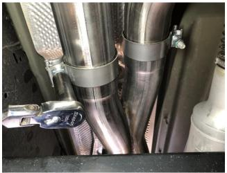
4. Locate the CORSA front crossover assembly and two 3.0" clamps. Position the 3.0" clamps onto the crossover inlet with the clamp hardware on the outside of each pipe, and the clamp nuts facing down. Insert the crossover onto the connector pipe and passenger head pipe outlets, making sure to have at least 1.75" of overlap at both slip fit connections, then snug the clamps using a 15mm socket and 3/8" ratchet, leaving them loose enough for later adjustment.
