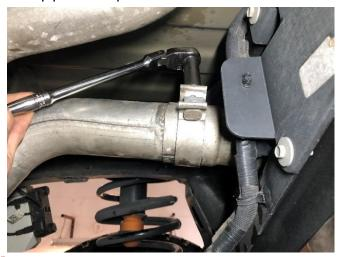
**4.** Using a 15mm socket and 3/8" ratchet, loosen the factory clamp securing the passenger side tailpipe.
