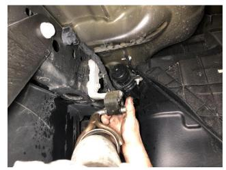
23. Locate the factory passenger side tailpipe. Insert the factory passenger tailpipe inlet through the chassis, and onto the CORSA passenger front tailpipe outlet as shown, making sure to have at least 1.75" overlap at the slip fit connection. Insert the factory passenger side tailpipe hanger into the exhaust grommet as shown.
