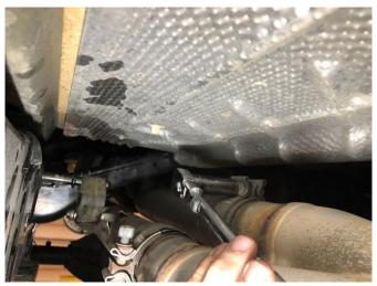
**8.** Using a 15mm socket and 3/8" ratchet, loosen the inner factory clamp securing the stock muffler section to the factory "Y" pipe.
