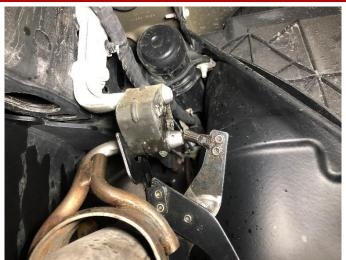
Using grommet pullers or similar device, remove the passenger side tailpipe hanger from the grommet.
