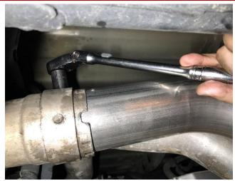
**24.** Snug the clamp at the slip fit connection of the factory passenger tailpipe inlet using a 15mm socket and 3/8" ratchet, leaving it loose enough for later adjustment.
