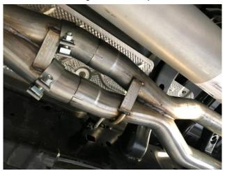
6. Locate two 3.0" clamps. Position both clamps onto the outlet of the front crossover assembly, such that both clamp nuts will be facing inwards below the piping (outwards when rotated above the piping) as shown. Insert the CORSA rear muffler (or Baja muffler delete) inlet onto the front crossover outlet; making sure to have at least 1.75" of overlap at both slip fit connections.
