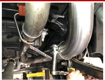
**25.** Snug the clamps at both slip fit connections from the muffler/muffler delete outlet using a 15mm socket and 3/8" ratchet, leaving them loose enough for later adjustment.
