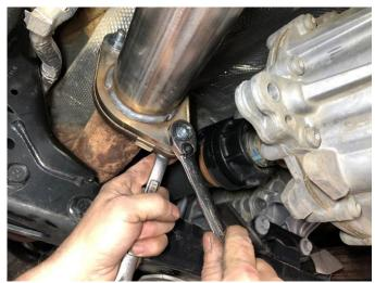
1. Locate the CORSA driver side head pipe assembly, and two each of the supplied M10 mounting bolts and nuts from the hardware kit. Install the driver side head pipe onto the flange from the driver side catalytic converter as shown and secure the flange with the M10 flange bolts and nuts, using two 15mm wrenches.
