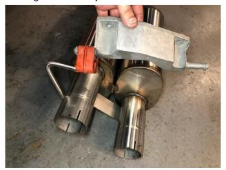
5. Locate the CORSA muffler (or Baja muffler delete) assembly and the rear muffler hanger mount set aside in REMOVAL STEP 10. Insert the rear muffler hanger into the grommet as shown; note the orientation of the rear muffler hanger mount when the grommet is installed. Once again, the use of a soapy water solution will aid in the installation of the hangers into the factory grommets.
