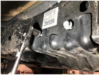
**13.** Locate the driver side skid plate behind the driver side catalytic converter. Remove the two bolts securing the side of the skid plate using a 16mm socket and 3/8" ratchet.
