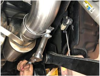
12. Locate the CORSA passenger front tailpipe and a 3.0" clamp. Position the 3.0" clamp onto the outlet of the muffler/muffler delete with the clamp hardware on the outer side (away from driveshaft) of the pipe and the clamp nut facing down. Insert the tailpipe inlet into the muffler outlet, making sure to have at least 1.75" of overlap at the slip fit connection, then snug the clamp using a 15mm socket and 3/8" ratchet, leaving it loose enough for later adjustment.
