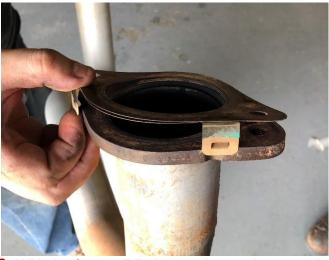
**18.** With the factory "Y" pipe section on the ground, remove both factory metal exhaust gaskets from the flange locations.
