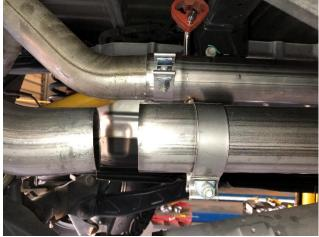
22. Locate the CORSA passenger front tailpipe and a 3.0" clamp. Position the 3.0" clamp onto the outlet of the muffler/muffler delete with the clamp hardware on the outer side (away from driveshaft) of the pipe and the clamp nut facing down. Insert the tailpipe inlet into the muffler outlet, making sure to have at least 1.75" of overlap at the slip fit connection, then snug the clamp using a 15mm socket and 3/8" ratchet, leaving it loose enough for later adjustment.
