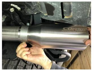
17. Locate both CORSA tip assemblies, and two 3.0" clamps. Identify the driver and passenger side tips by the CORSA etch location; the CORSA logo will face outwards and be upright on each side of the vehicle. Hold the driver side tip with the logo facing outwards, and slide a clamp onto the tip inlet, such that the clamp hardware sits to the top of the tip, and the clamp nut is facing outwards. Carefully install the CORSA driver exhaust tip onto the driver side tailpipe outlet.
