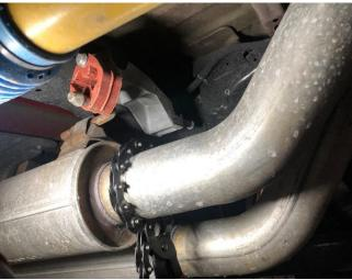
2. Using a chain cutter or similar device, cut the pipe on the CUT LINE, just behind the inner most factory muffler. NOTE: Carefully and thoroughly deburr the cut location on the driver side factory tailpipe. This step is critical for the Baja center section version of the CORSA exhaust to fit properly, as it reuses the factory tailpipes and tips.
