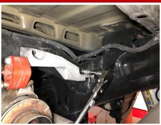
10. Remove the two nuts securing the rear muffler hanger mount using a 13mm socket and 3/8" ratchet. Set aside the two nuts to be reused during INSTALL STEP 8.
