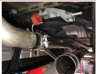
20. Locate the cut factory driver side tailpipe and a 3.0" clamp. Position the 3.0" clamp onto the outlet of the muffler/muffler delete with the clamp hardware on the outer side (away from driveshaft) of the pipe and the clamp nut facing down. Insert the cut factory tailpipe into the driver side muffler/muffler delete outlet as shown, with 1.75" of overlap at the slip fit connection.
