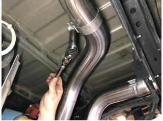
14. Insert the driver rear tailpipe inlet onto the driver front tailpipe outlet as shown, making sure to have at least 1.75" of overlap at the slip fit connection, then snug the clamp using a 15mm socket and 3/8" ratchet, leaving it loose enough for later adjustment.
