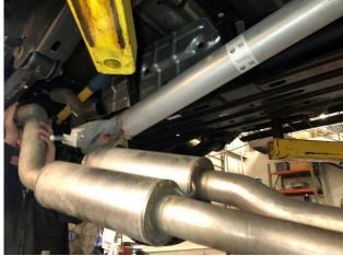
11. Carefully remove the factory muffler section by sliding it rearward to free it from the "Y" pipe, then moving it down and forward to free it from the vehicle.
