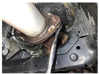
**15.** Remove the two bolts securing the passenger side "Y" pipe flange using a 16mm wrench.
