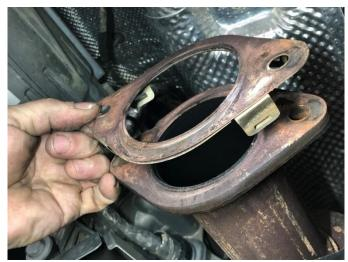
19. Install one of the factory exhaust flange gaskets as shown onto the passenger side factory flange on the outlet of the catalytic converter pipe, which is on the opposite side of the flange connection from the factory "Y" pipe.
