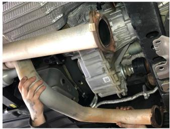
17. Carefully remove the "Y" pipe section by sliding it rearwards and then down and forward to free it from the vehicle.
