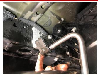
15. Locate the CORSA passenger rear tailpipe assembly and a 3.0" clamp. Position the 3.0" clamp onto the tailpipe inlet with the clamp hardware on the inside of the pipe, and the clamp nut facing down. Insert the passenger rear tailpipe hanger into the exhaust grommet as shown
