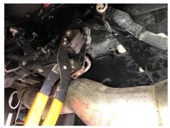
3. Using grommet pullers or similar device, remove the driver side tailpipe hanger from the grommet, then carefully remove the driver side tailpipe from the vehicle. NOTE: The use of soapy water solution will aid in the removal and later installation of the hangers from the factory grommets.
