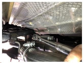
10. Snug the inner clamp at the muffler/muffler delete slip fit connection using a 15mm socket and ratchet. Leaving it loose enough for later adjustment.
