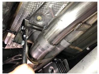
Snug the outer clamp at the muffler/muffler delete slip fit connection using a 15mm socket and ratchet, leaving it loose enough for later adjustment.
