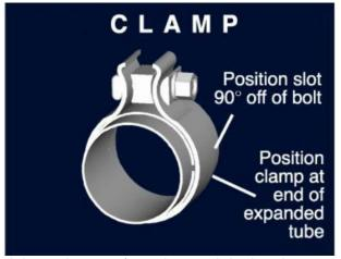
**NOTE:** Align all clamps so that the center of the clamp bolt is 90 degrees from the notch in the pipe.
