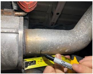
Identify the inner most factory muffler, closest to the driveshaft, located just in front of the rear differential on the passenger side of vehicle. Using a tape measure and a black marker, measure 1 3/4" off the rearward facing bottom edge of the muffler, then mark the pipe. This is the CUT LINE.
