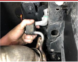
**21.** Insert the factory driver side tailpipe hanger into the exhaust grommet as shown.
