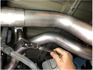
16. Insert the passenger rear tailpipe inlet through the chassis, and onto the passenger front tailpipe outlet as shown, making sure to have at least 1.75" of overlap at the slip fit connection, then snug the clamp using a 15mm socket and 3/8" ratchet, leaving it loose enough for later adjustment.
