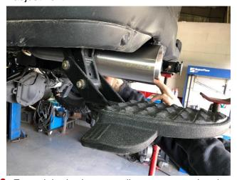
18. Extend the bed step to allow access to the clamp location on the tip inlet. Adjust the position and rotation of the tip to center the logo on the outer side of the tip, with the desired amount of tip reveal, making sure to have at least 1.75" of overlap at the slip fit connection. Secure the tip using a 15mm socket and ratchet, leaving it loose enough for later adjustment.
