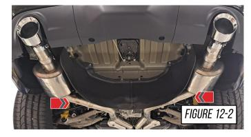
Make your final adjustments to the tips to ensure they are in a position you like. Once the desired positioning is achieved work from the front of the car to the back, tightening all the clamps fully and ensuring there is proper clearance of the chassis, and braces.
