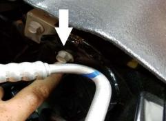
6 Mount J&L Oil separator to bracket with supplied screws, the fittings should be facing the driver side of the truck.
