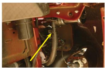
138. Cut 1-1/2" off the end of one of the supplied 4" x 36" x 90° elbow hoses.
