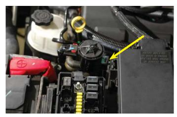
123. This is the charge air cooler pump and mounting hardware.
