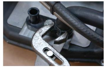
96. Connect the short end of the other modified 4" x 36" x 90° elbow hose to the left hand side charge air cooler hose barb behind the supercharger using a provided spring clamp. This hose will also route toward the right hand side of the vehicle.
