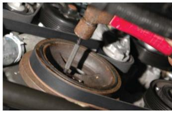
194. Install the OEM crank pulley bolt and torque to 129 ft. lbs.
