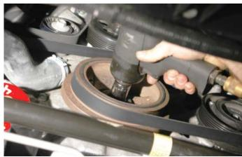
186. Install the provided drill guide using the provided crank bolt and torque to 40 ft. lbs. It's helpful to align the holes in the guide horizontally.
