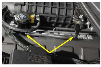
115. Install a 24" piece of the supplied 1/2" hose between the right hand side PCV barb in the supercharger lid and the right hand side barb of the oil separator valve.
