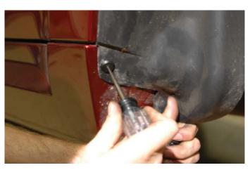
127. Remove the splash shield fender well from the vehicle and set aside to reinstall later.
