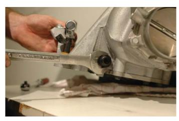
83. Install the PCV valve in the right hand side hole of the supercharger lid and tighten with 15/16" wrench.
