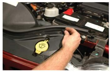
200. Find a place to loop the cable of the OBD port (a panel behind the port can be opened and the cable looped around the wire harness inside) and press the cover over the port.
