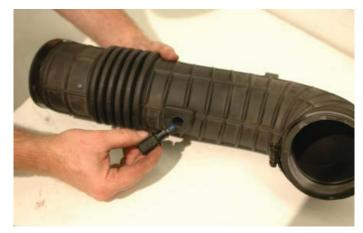
89. Lube the O-ring of the removed IAT sensor with the provided Lubriplate lubricant.
