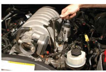
30. With the help of an assistant, carefully lift the OEM intake assembly from the vehicle. At this time if you didn't have success pulling the MAP sensor plug free, with the manifold moved slightly forward you should have an easier access to disconnect the sensor. Snake the brake booster hose around the existing water heater hoses as you pull the intake assembly out of the vehicle. Set aside as we will be using components later in assembly.
