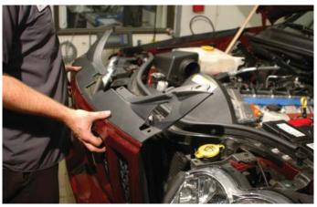
64. Cut strips of the supplied adhesive backed rubber and apply to the inside surfaces of the low temperature radiator mounting brackets, on top of the strips applied, cut and add the ½" adhesive backed rubber as shown.
