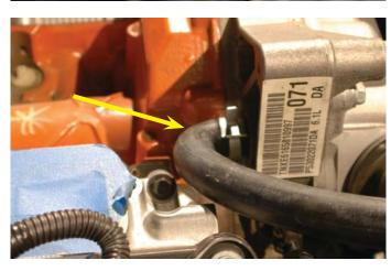
51. Route the hose toward the right hand side fender. Use the bolt hole at the front of the right hand side head near the water pump, add the supplied spacer, then the Adel clamp with the lobe up and pointed toward the rear of the vehicle, and the supplied bolt to anchor the heater hose as shown in this picture.
