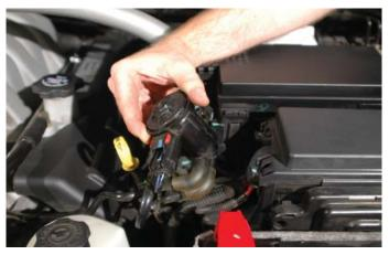
8. Open the cover of the forward fuse center just behind the battery on the left hand side of the engine compartment, and un-snap the hinges from their posts to remove the cover. Set aside for later usage.
