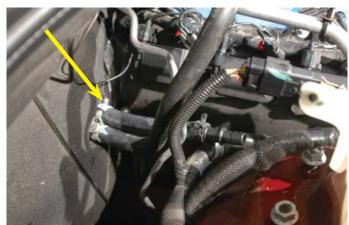
54. Cut the right hand side hose installed at the water pump to meet the coupling (hose mender) installed on the 7" hose just installed. Press onto the coupling and secure with a supplied spring clamp.
