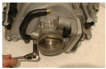
86. Inspect the installed throttle body O-Ring on the new supercharger inlet. If there is any nicks or damage to the O-Ring it must be replaced.
