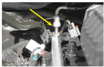
110. Pull on the fuel line; this should not be removable without using the fuel line removal tool. After verifying your connection, snap on the fuel line safety clip.
