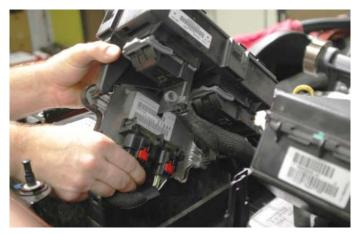
120. Install the forward fuse center onto the three fuse center mounting bracket posts. An audible click is heard when locked in place.
