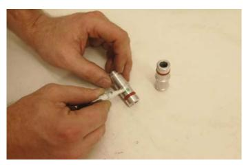
47. Use your fingers to press one of the prepared barbs into the right hand side hole in the back of the water pump that was vacated by the right hand side hard line heater pipe that ran under the OEM intake manifold.
