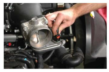
105. Plug the EVAP sensor tube onto the inlet on the supercharger inlet as shown.
