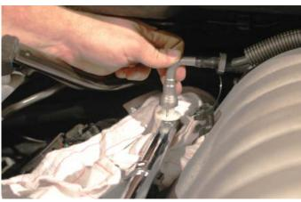
29. Remove the ten 8mm bolts holding the OEM intake manifold to the heads.
