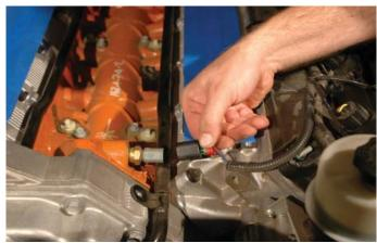
42. Use a large flathead screwdriver to carefully lever the heater hard line barb from the water pump on the left hand side using the water pump as a fulcrum.
