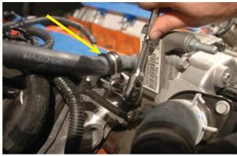
52. Install the supplied ¾" -5/8" coupling (hose mender) in the supplied ¾" x 7" section of hose. Secure in place with a supplied spring clamp.
