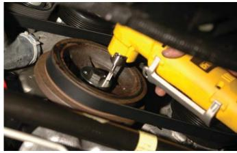
190. Remove the temporary crank pulley bolt and drill guide.
