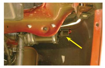
153. Tuck the yellow wire into the split loom covering the red wire from the relay. Route the two wires into the engine compartment over to the rear fuse center on the engine side. Tuck a loop of the harness up into the forward cavity of the fuse center, and pull the yellow wire out of the split loom at the peak of the loop. Remove the nut from the positive post of the fuse center.
