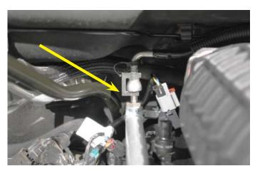
111. Extend the 'lobe' of the notch in the left hand side coil pack cover approximately 1" further toward the rear of the cover and press in place over the coil packs in the original location. This modification is to create clearance with the oil separator drain hose to be installed next.
