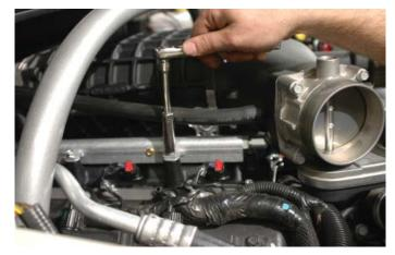
141. Attach the supplied charge air cooler reservoir mounting bracket to the forward right hand side fuel rail mounting boss location, re-installing the fuel rail mounting bolt. Tighten securely using a 10mm wrench.
