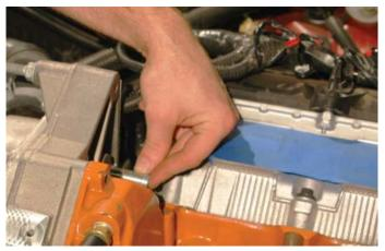
48. Use your fingers to press the other prepared barb into the left hand side hole of the water pump that was vacated by the removal of the left hand side hard line heater pipe that ran under the OEM intake manifold.
