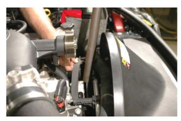
171. Remove the top water pump bolt using a 13mm wrench.
