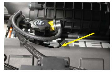
112. On the left hand side below the windshield cross brace is an existing stud pointing down. Use the provided nut to attach the provided bracket to the stud and tighten with a 10mm wrench.
