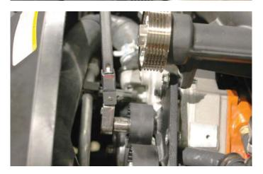
179. Torque the second water pump bolt (finger-tightened earlier) using a 13mm wrench and torque to 20 ft. lbs. Always verify your torque wrench settings.
