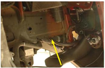
136. Connect the short end of the other modified 4" x 60" x 90° elbow hoses to the left hand side hose barb of the charge air cooler low temperature radiator and route over toward the right hand side to parallel the hose just installed into the wheel well. Secure in place with a provided spring clamp.
