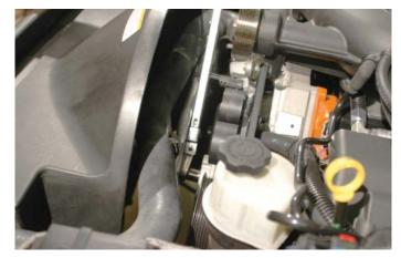
181. Install the drive belt on the engine using the belt routing diagram located on the last page of these instructions as a guide. Spring the tensioner using a 3/8" ratchet or breaker bar (we use a pipe for ease of leverage on a 3/8" ratchet).
