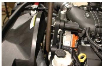
182. Replace the AC mounting bracket back on the post in front of the engine.
