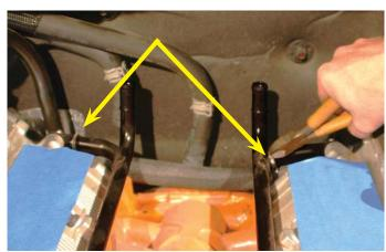
38. Use a 10mm wrench to remove the studs holding the two heater hard lines to the back of the heads.
