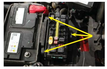
121. Replace the rear fuse center on the four fuse center mounting bracket posts. Ensure they click into place.
