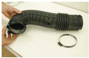
166. This is the air tube components, including the two clamps removed from the OEM unit.
