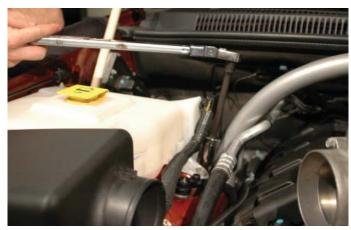
118. Install the fuse center mounting bracket using the original three nuts and tighten using a 10mm wrench.
