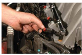
23. Disconnect the MAP sensor from behind the air intake manifold on the right hand side behind the OEM manifold. If you cannot get this unplugged easily, you will have another chance while you are removing the OEM manifold a little later in the instructions.
