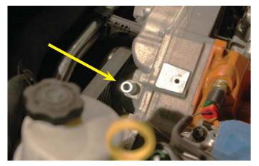
49. Remove the stock center-most heater hose from the firewall hose barb on the right hand side of the engine compartment.
