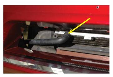
135. Continue to route the hose around the radiator support frame, in and over the lower radiator hose and up into the engine compartment on the right hand side over the coil packs back toward the rear of the vehicle.
