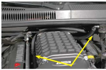
116. Install a 42" piece of the supplied 1/2" hose between the right hand side barb on the supercharger inlet and the left hand side barb of the oil separator valve.
