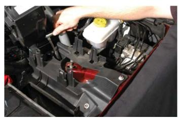
119. Re-connect the two forward fuse center plug connections.
