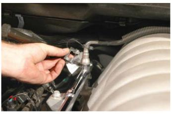
28. Use shop rags to catch residual fuel and the fuel line removal tool to disconnect the fuel line from the right hand side fuel rail. First press the fuel line further onto the fuel rail barb, then push the fuel line removal tool into the fuel line to release the locking clip. Now pull the fuel line free. We recommend plugging the fuel line and capping the fuel rail barb. Clean up residual fuel using shop rags and dispose of the contaminated rags properly.
