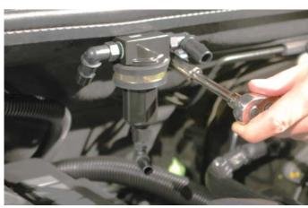
114. Trim the 3/8" hose to fit between the oil separator valve and oil fill spout barb and install between the two, no clamps are necessary.
