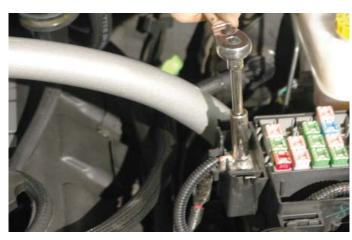
155. Remove the 25A fuse #43 for the fuel pump from the rear fuse center. Verify using the owner's manual that you are removing the coil-actuators fuse.
