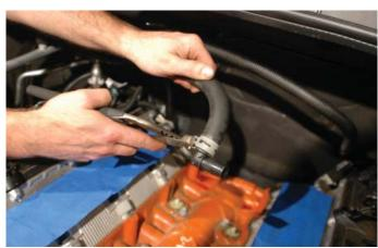
58. Attach the supplied 5/8" x 48" hose to the left hand side barb installed on the water pump using a supplied spring clamp.
