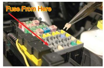
156. Add the fuse tap supplied to one leg of the 25A fuel pump fuse.
