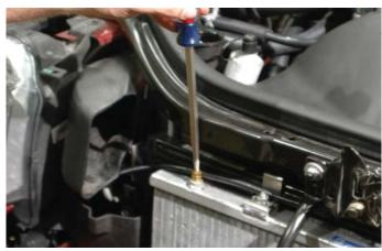
198. Fill the radiator back up with the fluid drained earlier. Be sure to incorporate a filter in case any debris contaminated your fluid. Top off as necessary.
