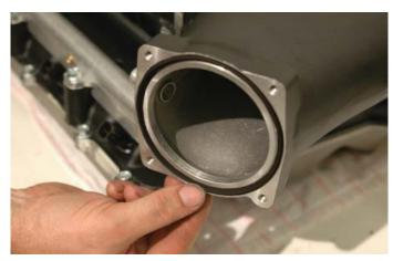
87. Install the throttle body on the new supercharger intake with the motor pointing down. Use the stock bolts removed from the OEM manifold and torque to 106" lbs. Verify your torque wrench settings.
