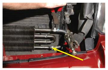
69. The existing power steering cooler plastic mounting tabs will have to be removed. We found the easiest solution was to use a saw blade to cut the tabs off of the mounting plate.
