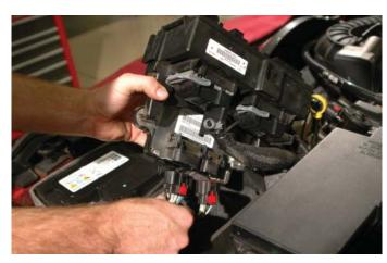
11. Again use a small screwdriver to release the locking clips of the rear fuse center located just forward of the brake reservoir. Pull the rear fuse center up off the mounting posts and push it over toward the engine with the forward fuse center.
