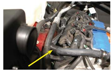
56. Cut about 1-1/2" from the end of the other heater hose at the firewall that used to run to the left hand side hard line running under the OEM intake manifold.
