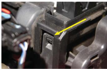
10. Lift the forward fuse center and unplug the two wire harness plugs from the bottom of the fuse center. Pull the fuse center up and over toward the engine.
