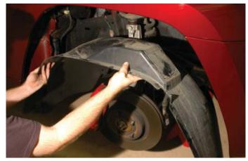
128. Mark a hole <sup>3</sup>/<sub>4</sub>" down from the center of the vertical-to-horizontal bend of the fender cross brace.
