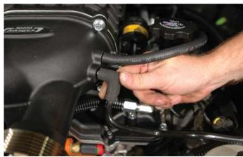
106. Remove the stock brake booster hose from the OEM intake manifold.
