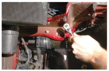
132. Roll the clamps forward and up after tightening and twist the pump to keep the discharge barb pointing down.
