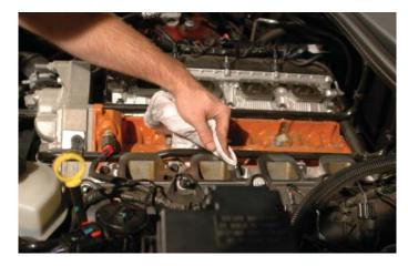
33. Use tape or shop rags to cover the exposed ports to prevent contamination.
