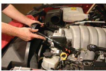
26. Disconnect the EVAP hose from the left hand side of the manifold, just behind the throttle body.
