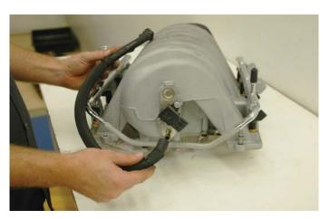
107. Remove the brake booster valve from the end of the hose and re-connect the valve to the opposite end of the hose by the "J" bend.
