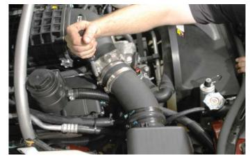
169. Near the front-center of the engine is a plastic mount anchoring the AC hard line to a stud. Pry this mount off the stud using a large flathead to get a little more room.
