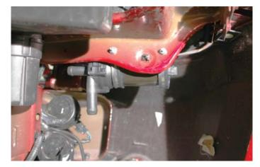
133. Cut 2-1/4" off the short end of the two supplied 4" x 60" x 90° elbow hoses.
