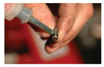
193. Insert the pins in the prepared holes and tap in using a punch. Make sure the pins are all the way in, the crank pulley bolt should not be able to touch the surface of the pin.
