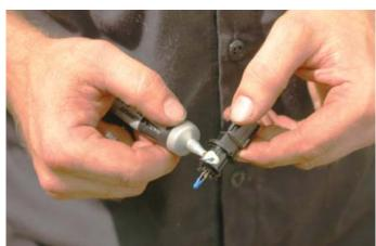
90. Flip the supercharger assembly upside down onto clean shop towels. Remove the bolt and mounting bracket over the IAT grommet temporarily. Press the IAT sensor into the grommet in the bottom of the supercharger assembly with the notch in the stop ring pointing toward the mounting bolt hole. Secure in place with the tongs of the mounting bracket and bolt.
