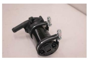
131. Secure the pump as described using the supplied nuts on the rear side of the fender cross brace. The discharge barb of the pump is to point down with the inlet barb of the pump pointing toward the left hand side of the vehicle. Tighten in place using a 10mm wrench.
