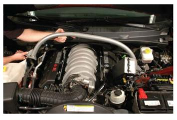
16. Remove the two HEMI coil covers from the vehicle by pulling up to unsnap from the mounting posts.
