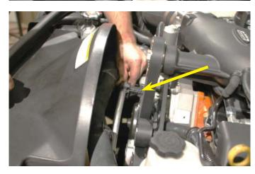
183. Remove the air box end of the hose from the OEM PCV plastic line and replace with the provided 4" section of 5/8" hose. Connect the remaining OEM hose end to the front oil fill spout hose barb and the new hose end to the air box end and air box. Secure to the air box using the provided spring clamp.
