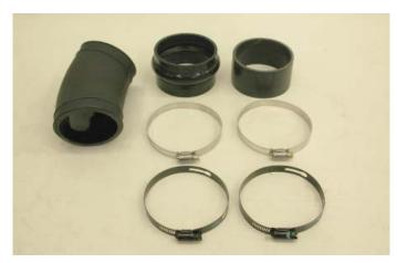
167. Mark and notch the supplied 'hump' hose to go past the two fins on the top of the OEM air box.
