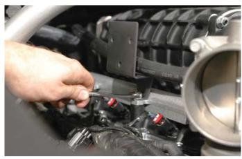
142. Modify the OEM right hand side coil pack cover to create clearance with the throttle body, slide under the charge air cooler reservoir mounting bracket and press onto the mounting studs locking in place.
