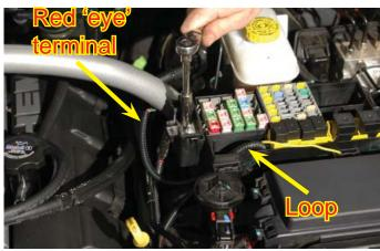
154. Replace the nut incorporating the "eye" on the end of the red wire of the relay harness.
