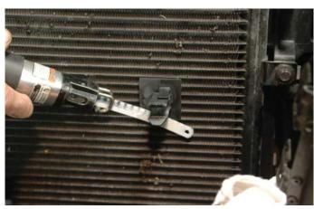
70. There is an existing threaded hole in the top surface of the bumper support on the left hand side. Use a drill motor and drill bit to open this hole to ½".
