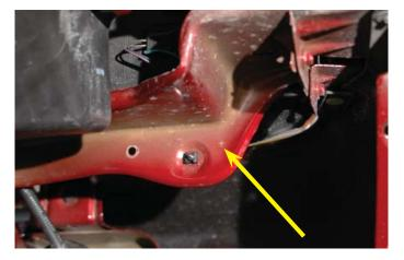
129. Drill a ¼" hole at the mark for an charge air cooler pump mounting clamp.
