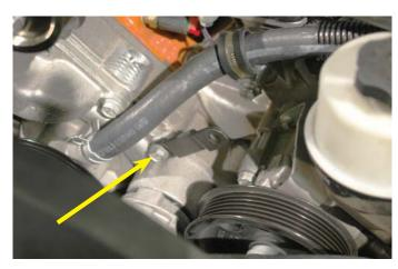
175. Attach the supplied idler bracket to the top water pump bolt location and the supercharger pulley support using the provided bolts. Torque to 20 ft. lbs.
