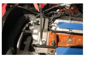
43. On the right hand side the heater hard line needs to be pulled toward the rear to remove it from the water pump. Use the large screwdriver with the head as a fulcrum to lever the hard line free from the water pump.
