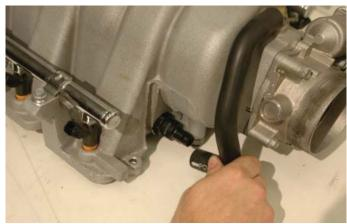
82. Use a 15/16" wrench, remove the PCV valve from the stock intake manifold.
