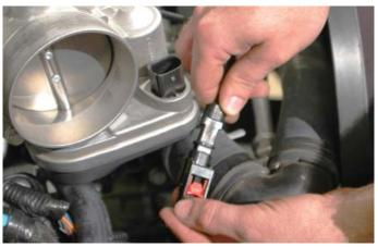
104. Plug in the throttle body connection.
