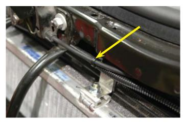
152. Connect the charge air cooler relay harness plug to the receptacle on the charge air cooler pump.
