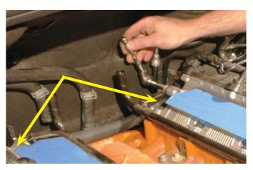
39. The left hand side heater hard line has two additional mounting bolts. Use a 10mm wrench to remove the center mounting bolt from the middle of the valley.
