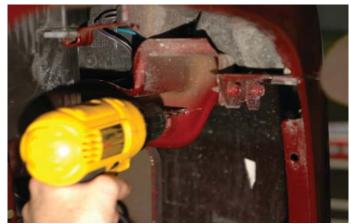
130. The pump will mount to the forward side of the hole you just drilled and the existing hole toward the center in this configuration. Note that the spacers will be against the cross brace, the clamp comes next with the lobes pointing down and forward.
