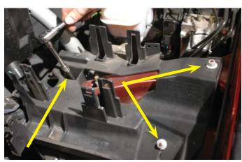
14. You now have access to the left hand side bolts holding the strut tower brace in place. Use an 18mm wrench to remove the nuts securing the strut tower brace in position (two each side). We used an impact wrench but this is not necessary.
