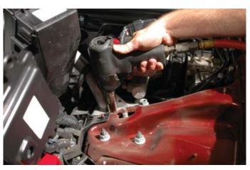
15. Pull up on the strut tower brace to pull it off the studs. On the left hand side, the mounting flange will hit the bottom of the brake cylinder. Pull the brace completely off the right hand side, and angle the brace to the rear to gain clearance to further pull the strut tower brace from the vehicle. Set aside for later use.
