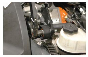
177. Add the supplied nut to the back of the idler pulley bolt securing the idler bracket brace using a 15mm wrench.
