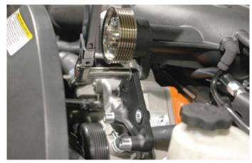
176. Add the idler pulley with the supplied longer bolt to incorporate the bracket brace installed earlier. Use a 15mm wrench and torque to 40 ft. lbs.
