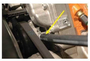
59. Use the bolt hole on the front of the left hand side head, the supplied spacer, then Adel clamp and bolt to anchor the hose you just installed to the engine. The lobe of the Adel clamp should be pointing up and toward the front of the vehicle.
