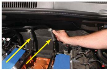
36. Use a 10mm wrench to remove the nuts holding the ground wires and ground sensor from the studs anchoring the heater hard lines to the back of the block. There are ground wires on both the left hand side and right hand side. Pull these wires and the ground sensor from their studs.
