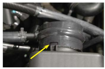
168. Install the notched hose in place on the air box. Slide the other hose completely onto the new air tube throttle body end. Press the air box end of the air tube into the receiving end of the hump hose...rotate the air tube to fit and slide the straight hose onto the throttle body. Tighten all clamps securely.
