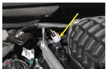
102. Connect the eight fuel injector plugs. Ensure that they clip securely in place.
