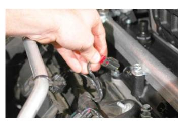
103. The IAT extension harness should be exiting below the supercharger intake manifold assembly on the right hand side of the engine. Connect the extension to the existing IAT plug and tuck the wires under the throttle body upon completion.
