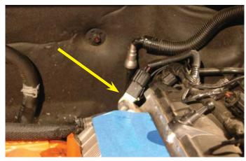
45. Replace the right hand side ground wires to the head using the original stud. Make sure you have accounted for all the wires.
