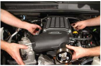
100. Torque the supercharger mounting bolts to 106" lbs. using a center-out, crisscross pattern. Verify your torque wrench settings.
