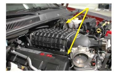
117. Re-install the strut tower brace using the original nuts, an 18mm wrench and torque to 70 ft. lbs.
