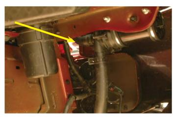
140. Remove the forward right hand side fuel rail mounting bolt using a 10mm wrench.
