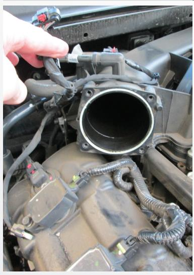
Now with the stock throttle body removed make sure to clean factory o-ring gasket as it will be re-used.
