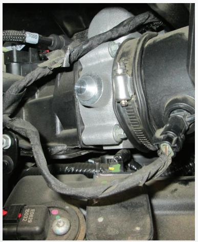
Re-install throttle body control plug, air temperature plug and intake tube back on to BBK throttle body.
