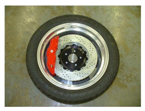
• When installing rotors on any Baer Products be sure to follow the direction of rotation indicated on
