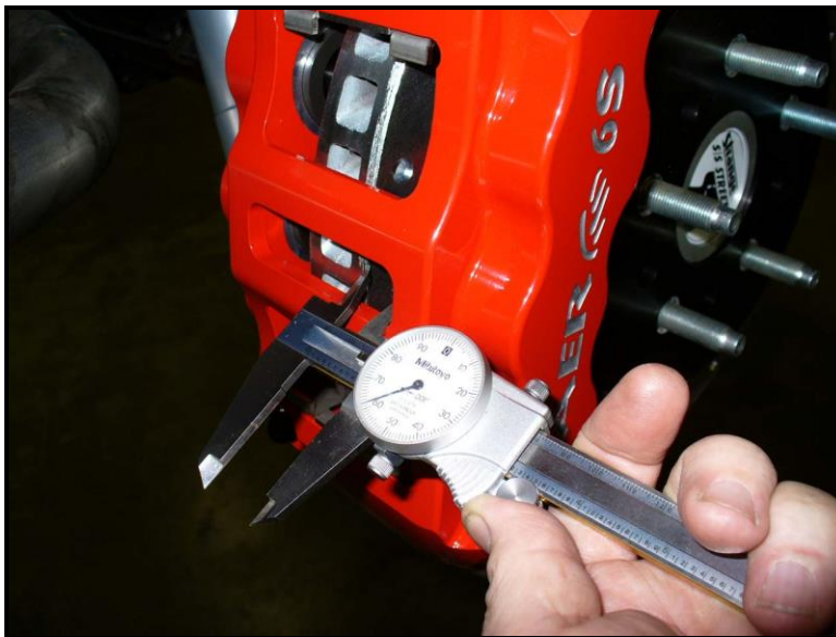
Figure 2: Obtaining gap measurements (6S Caliper shown)
