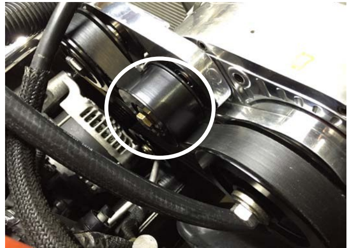
Idler Pulley Installed
