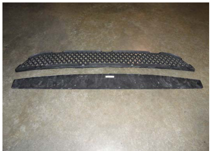
Mesh Grill Insert After Trimming
