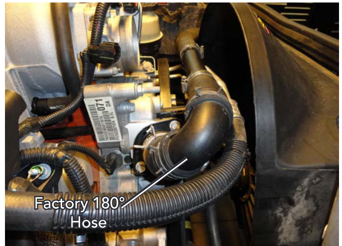
Upper Radiator Hose Installed
