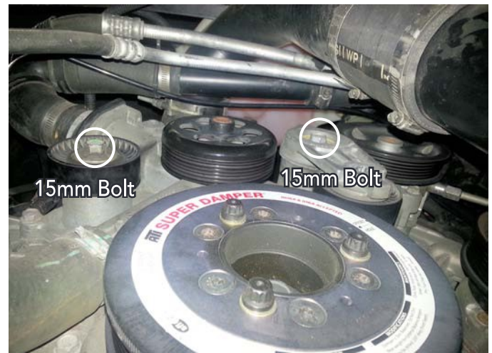
Factory Tensioner and Idler Pulley
