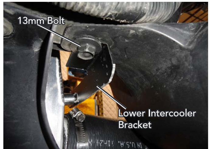
Lower Intercooler Bracket Installed (Passenger Side)
