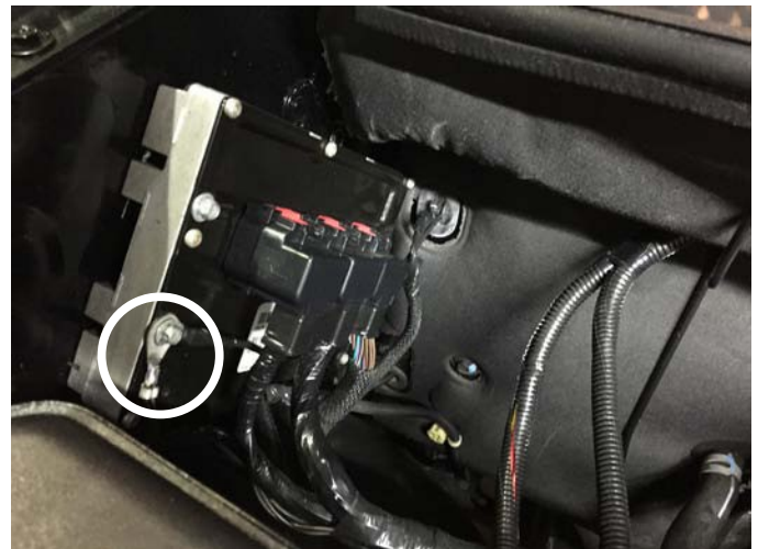
Ground Wire Attached
