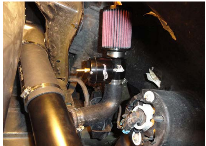
ProFlow Assembly Installed
