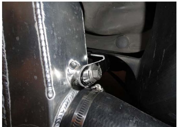
Lower Intercooler Bracket Installed (Driver Side)
