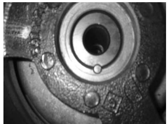
Crank Pulley Pinned to Crankshaft
