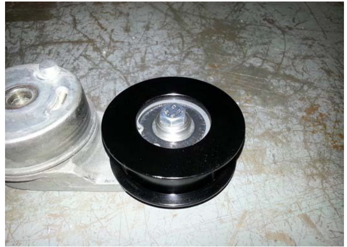
Shouldered Pulley Installed on Tensioner
