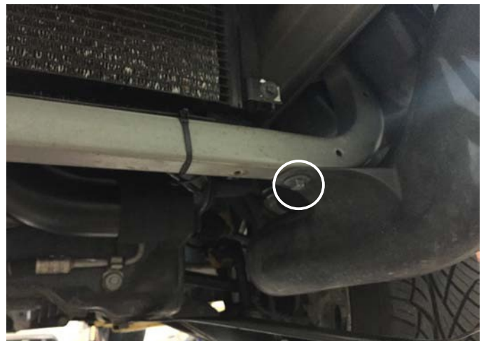
Brake Duct Bolt
