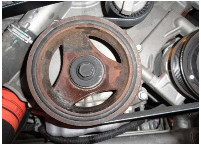
Factory Crank Pulley and Bolt
