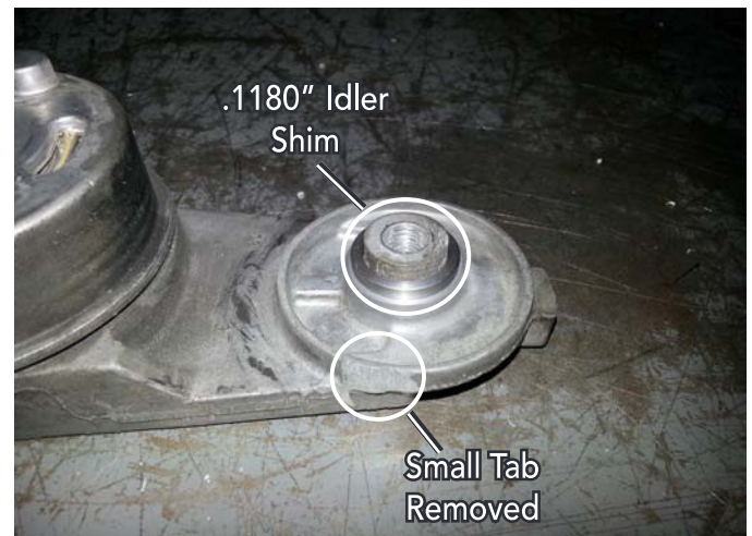
Idler Shim Installed / Tab Ground
