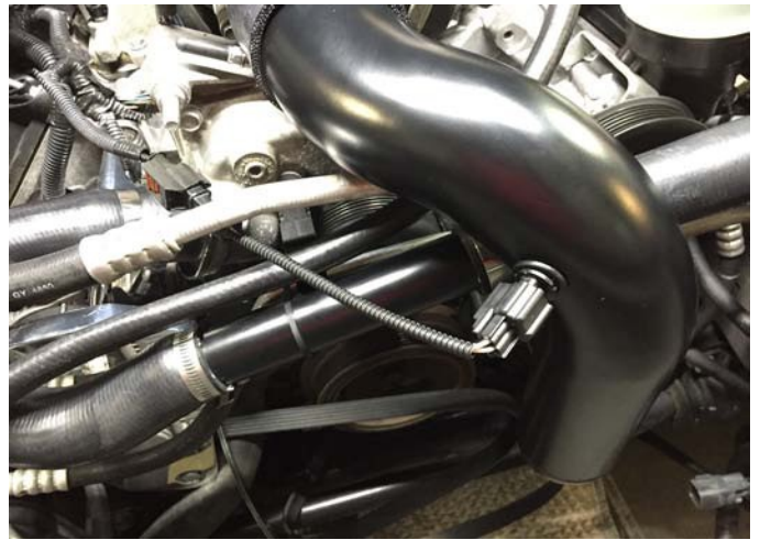
IAT Extension Harness Installed
