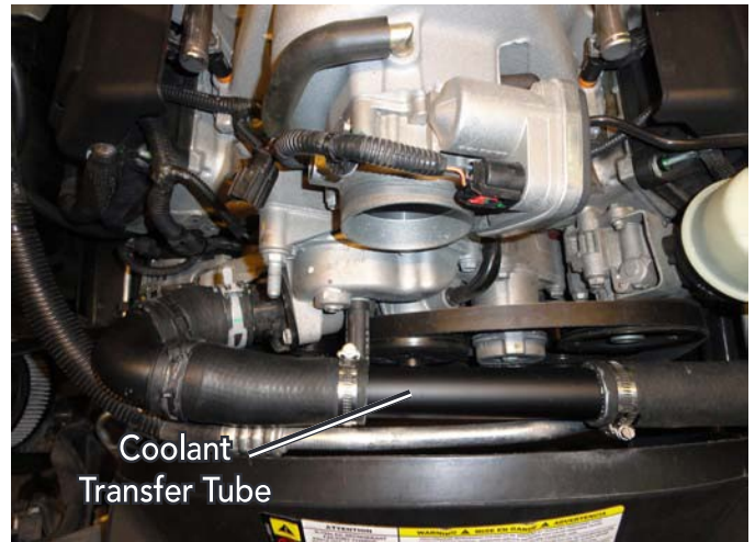
Coolant Transfer Tube Installed
