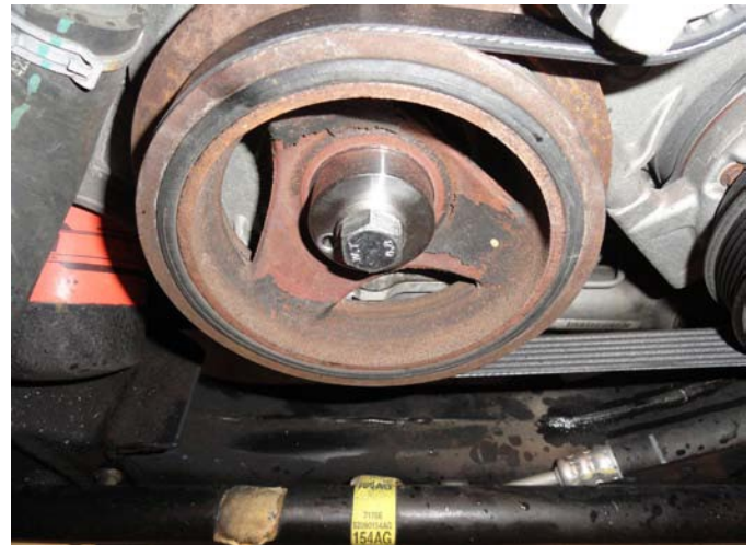
Drill Jig Installed
