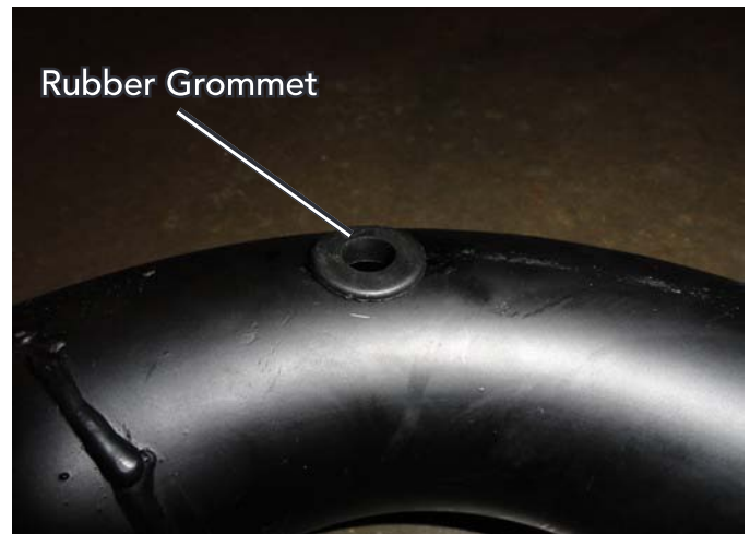
Rubber Grommet Installed Into Tube #330
