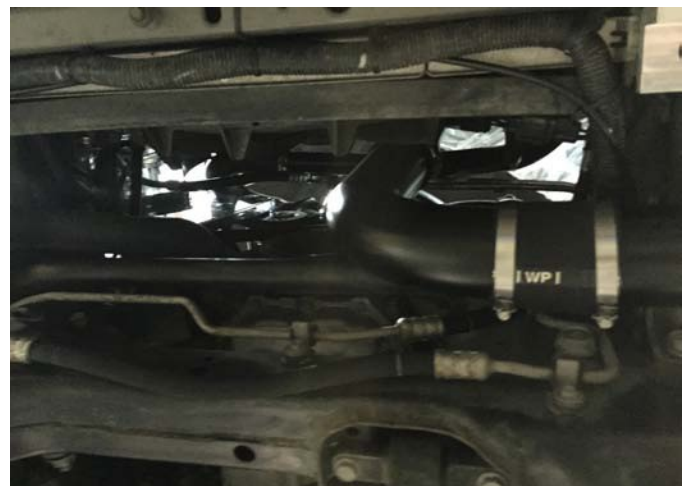
Tube #332 Routed To Throttle Body
