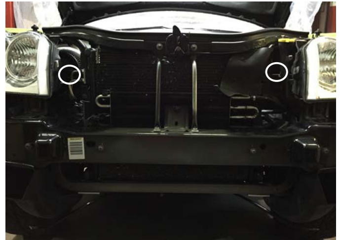
Radiator Hold Down Bolts
