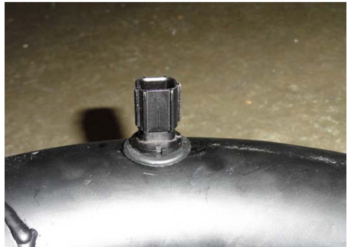
Intake Air Temp Sensor Installed
