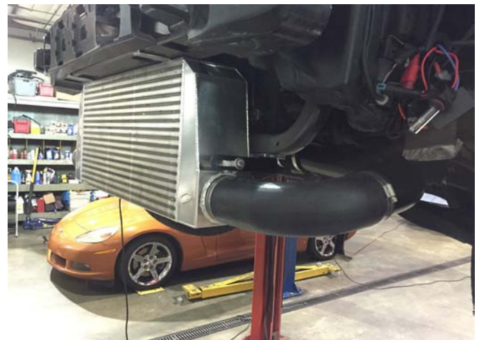
Tubing Out Of Intercooler Installed
