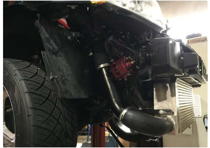
Tubing To Intercooler Installed
