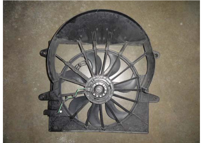
Factory Fan Assembly Removed
