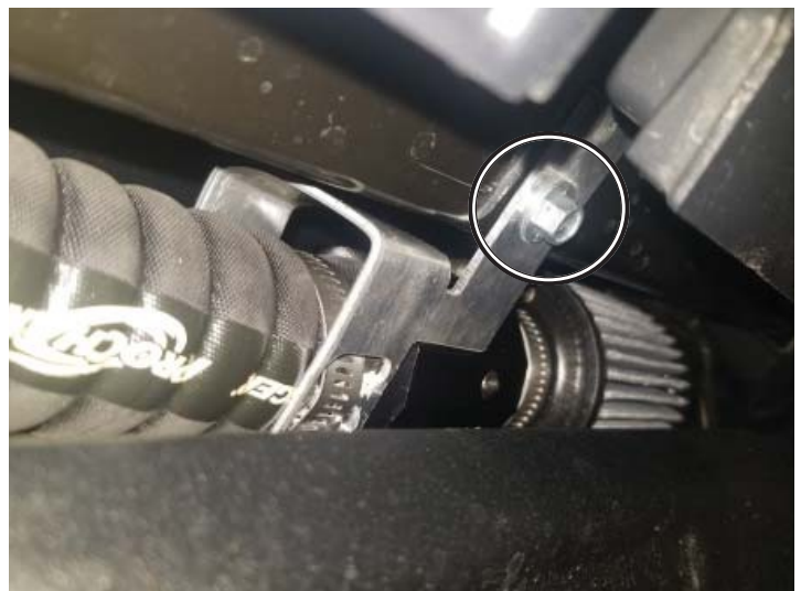
Surge Valve Installed
