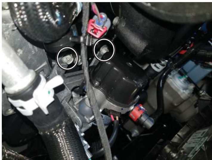
Air Pump Mounted
