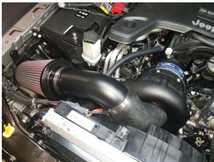
Air Inlet Installed
