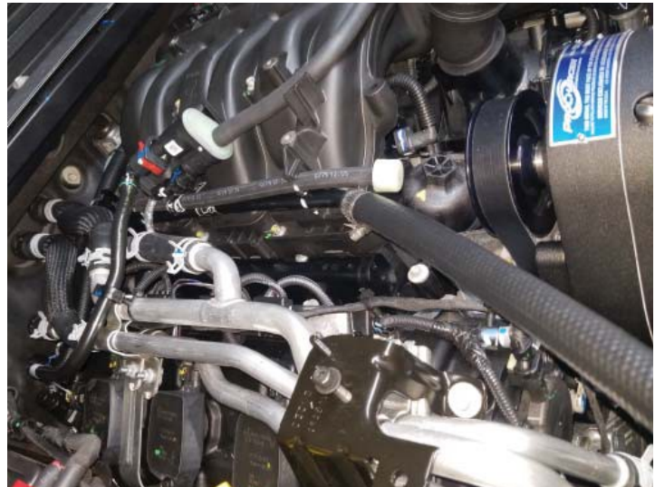
Hard PCV Line Trimmed
