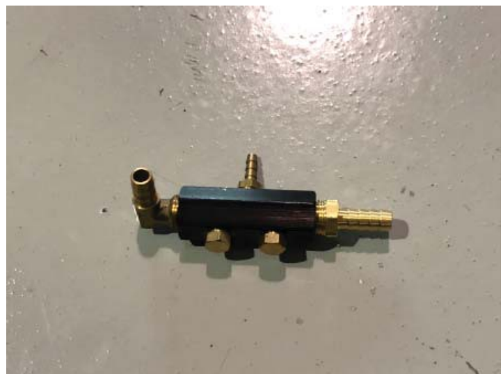
Vacuum Manifold Assembled
