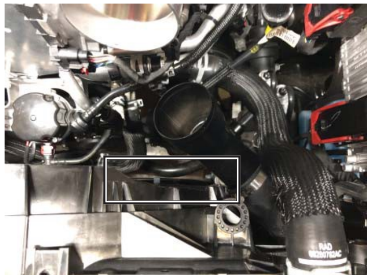
#372 Tube Installed / Fan Shroud Trimmed
