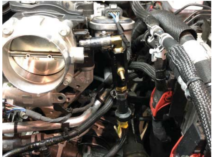
Vacuum Manifold Installed
