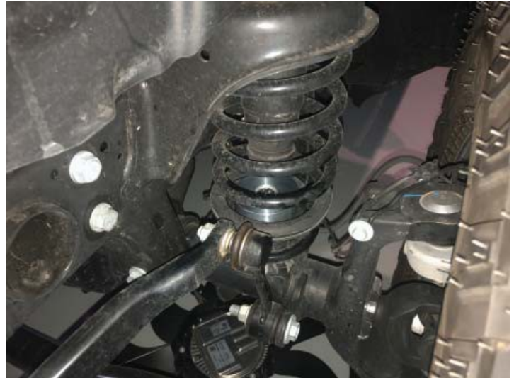
Bump Stop Installed
