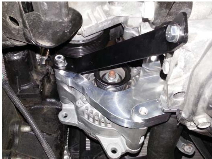
Alternator Brace Installed
