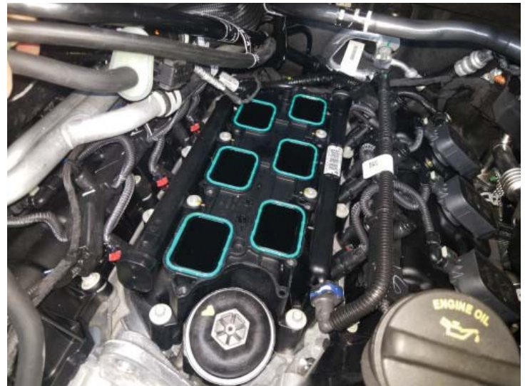
Intake Manifold Removed
