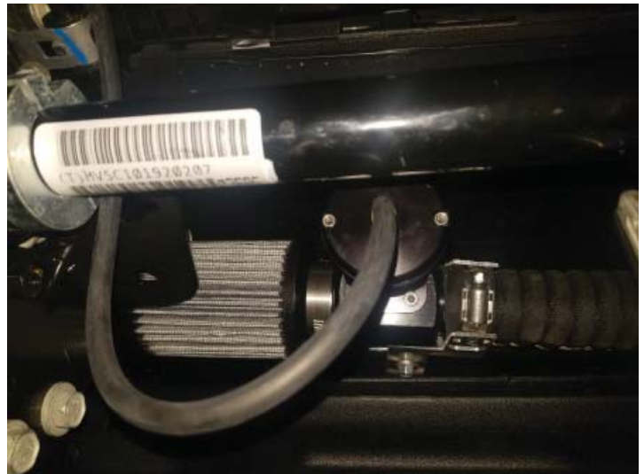
Surge Valve Installed
