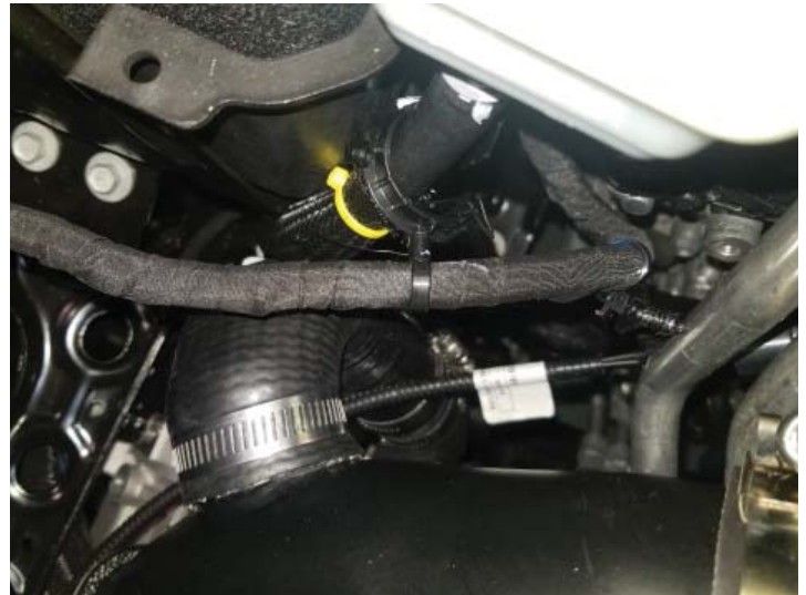
Moulded Rubber Hose Installed
