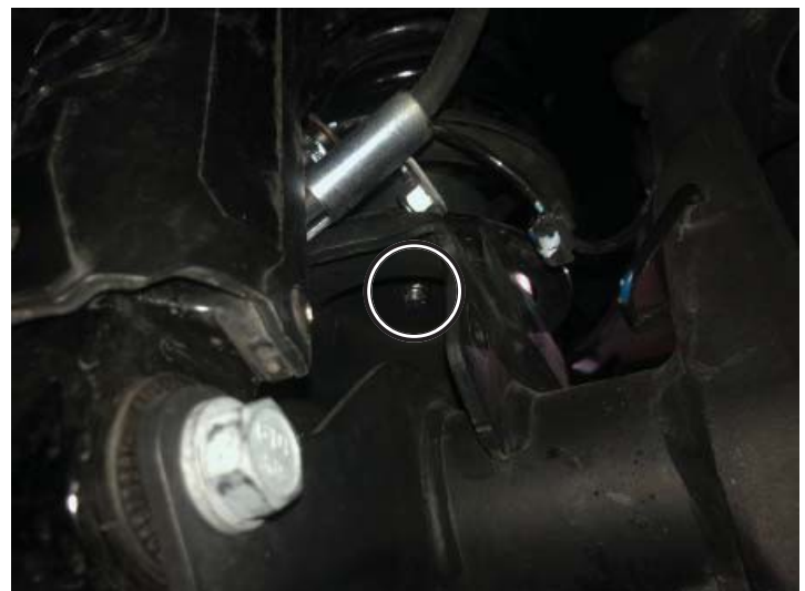
Bump Stop Nut Installed
