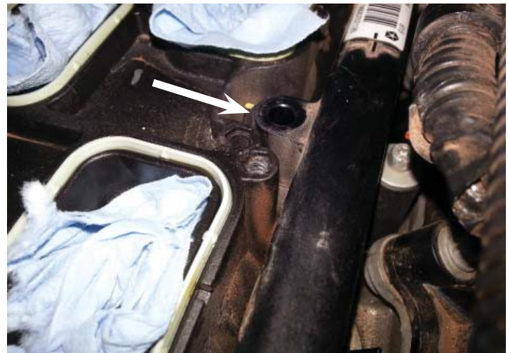
Fuel Rail Flush With Manifold
