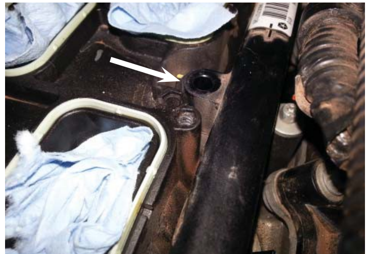
Fuel Rail Flush With Manifold
