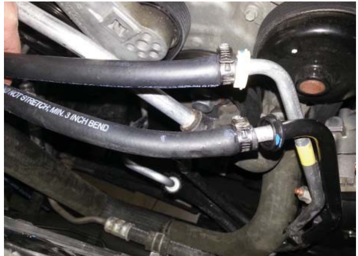
New Transmission Cooler Lines
