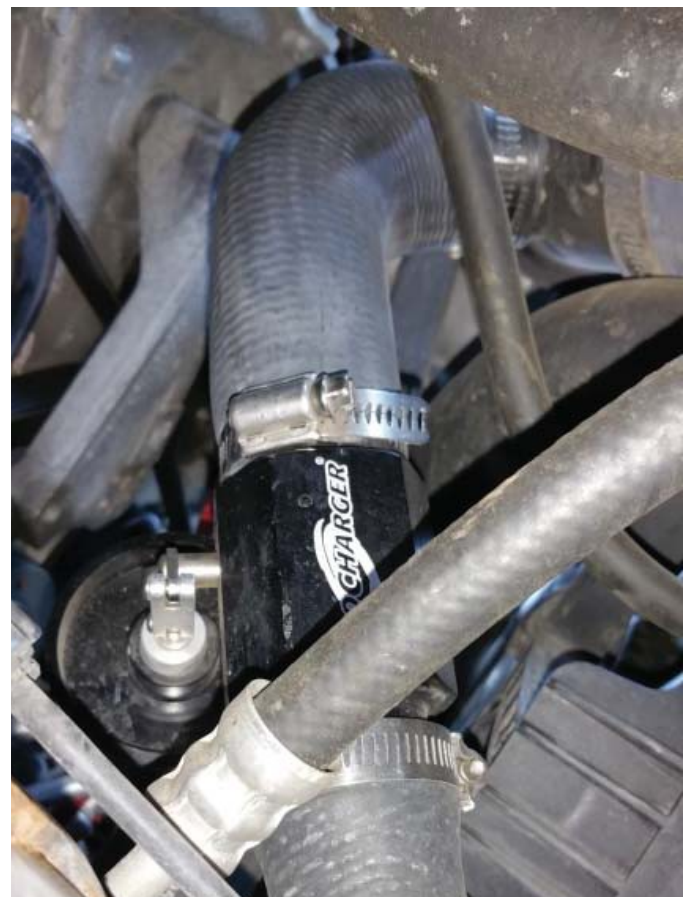
Surge Valve Installed
