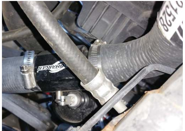
Short End Of Rubber Hose Installed
