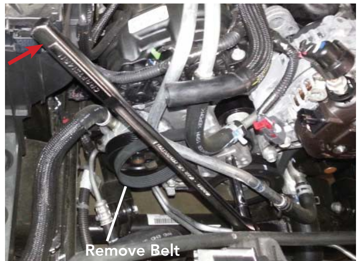
Compress the Tensioner and Remove Belt
