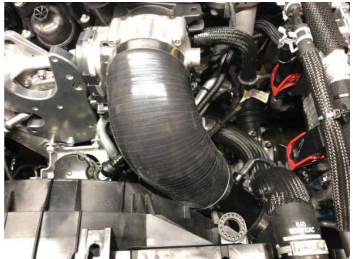
Throttle Body Tube Installed
