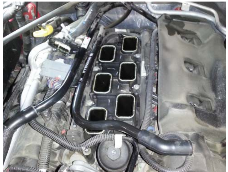
Intake Manifold Removed
