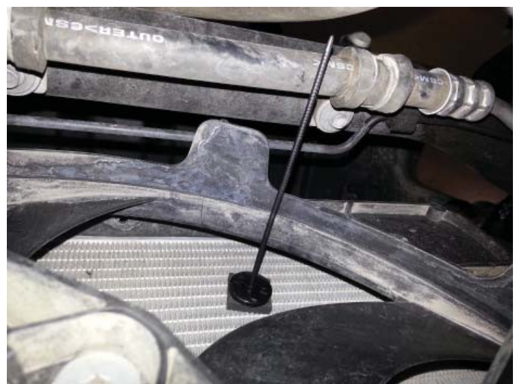
Cooler Mounting Rods Through Radiator
