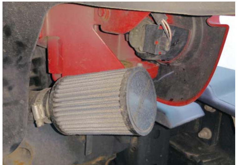
Filter Installed Onto Surge Hose
