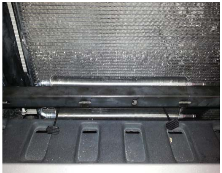
New Transmission Cooler Mounting Location
