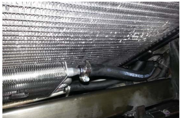
Transmission Lines Connected to New Cooler
