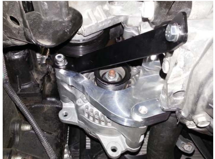
Alternator Brace Installed
