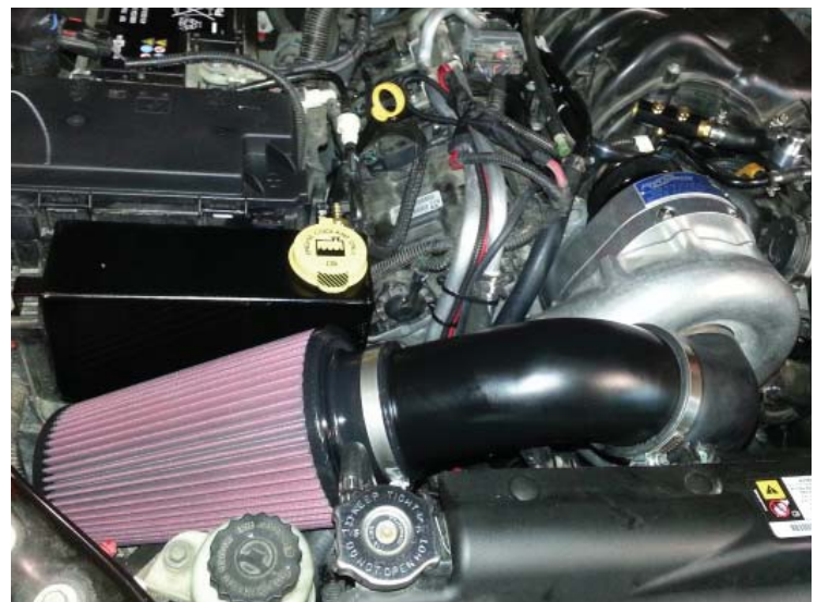
Inlet Tube Installed
