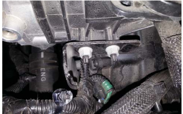
Manifold Front Bracket Nuts
