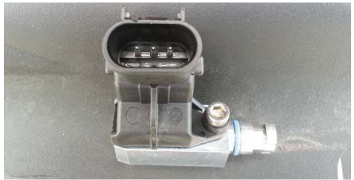
MAP Sensor Installed On Adapter
