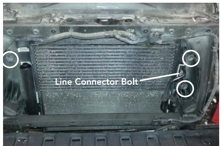
Transmission Cooler Bolts
