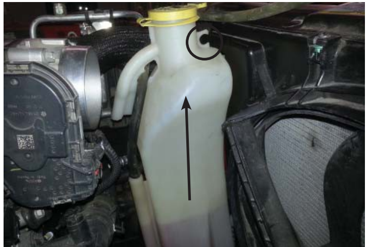
Coolant Overflow Reservoir
