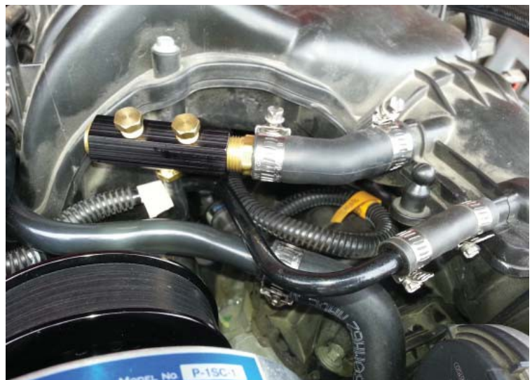
Vacuum Manifold Installed
