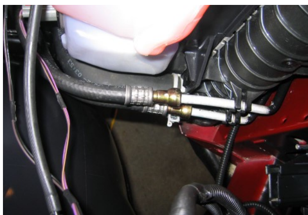
Main Water Line Clamps
