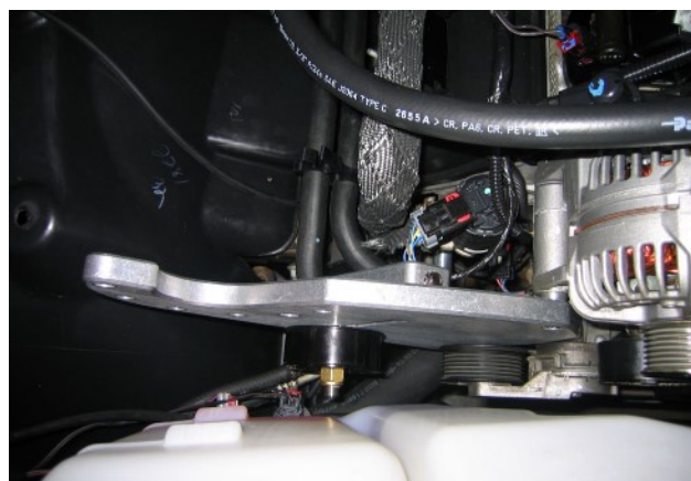
Main Bracket Installed
