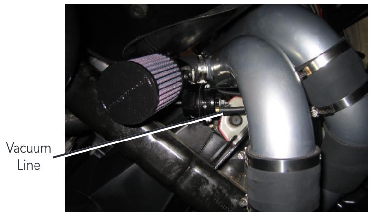
ProFlow Unit Installed
