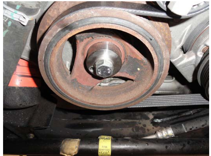
Drill Jig Installed
