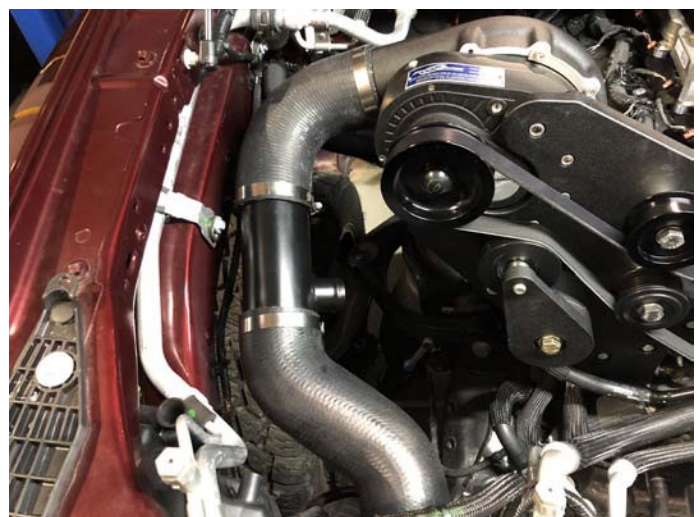
Tubing To Supercharger Installed
