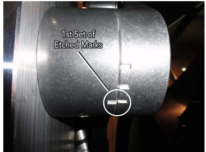
Proper Tensioner Position (View From Below)
