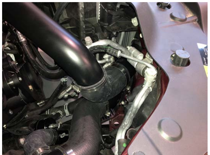
Tube #030 & 90° Rubber Elbow Installed
