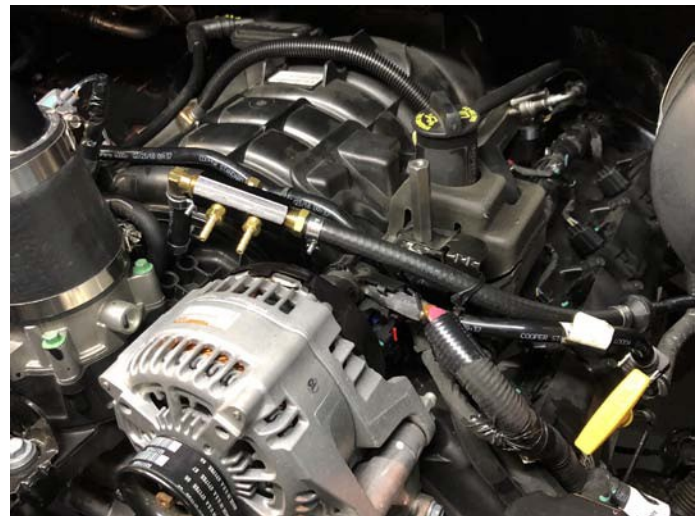
Vacuum Manifold Installed
