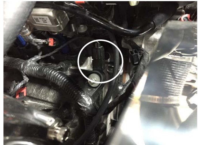
Ground Attached To Valvecover
