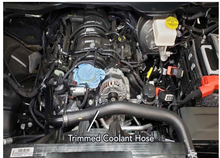
Upper Coolant Hose Installed
