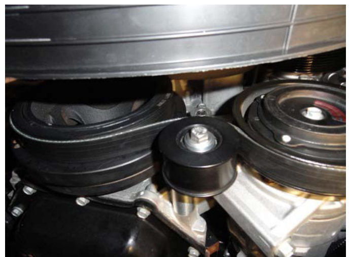
Idler Pulley Installed
