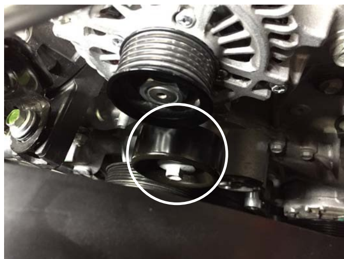
Idler Pulley Replaced
