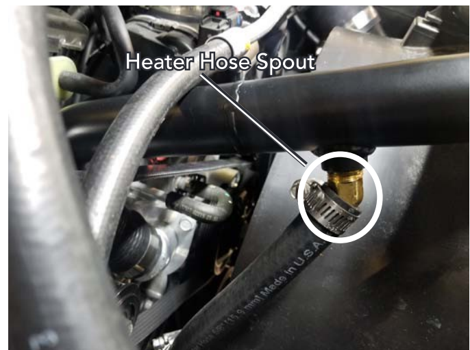
Transfer Tube Installed
