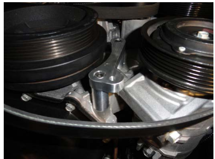
Idler Bracket Installed
