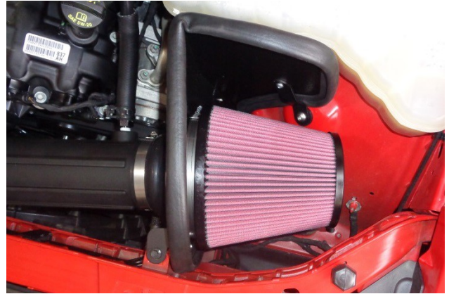
28. Place clamp (2) on air filter (1), install filter on filter adapter and tighten clamp.
