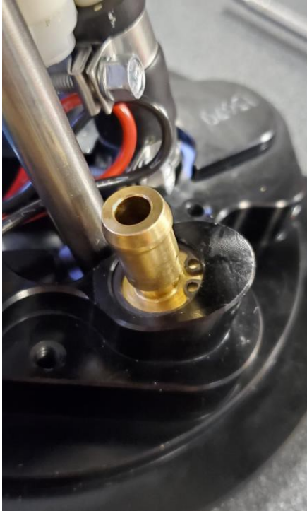
Fig 1: Barb installed into return port and retained with lock ring.
