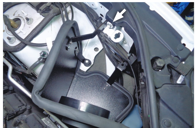
18. Install assembled heat shield into vehicle by pushing grommets (x2) onto pins. Re-install stock bolt (removed step 13) onto vehicle mount through bracket.
