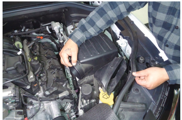
11. Pull airbox up sharply to release it from its mount grommets then remove it from engine compartment.
