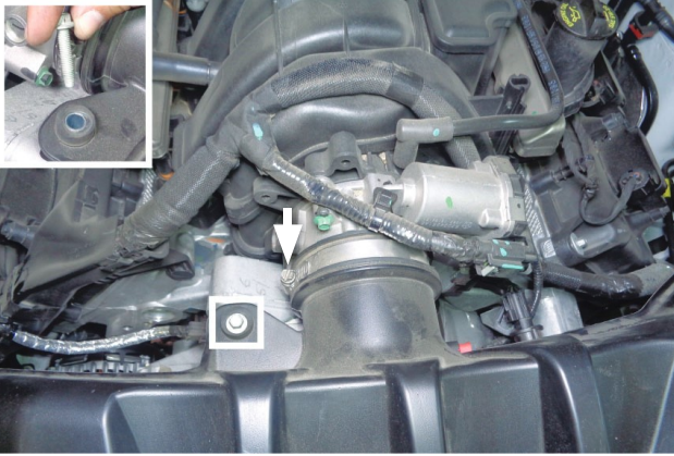
7. Loosen screw clamp holding resonator to throttle body then remove screw on resonator.
