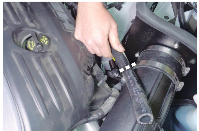
29. Route hose over to barbed elbow then trim to fit.
