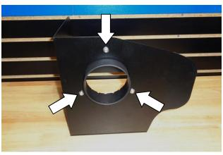
15. Assemble the air filter adapter (3) to the heat shield (4) using M6 screws (8), lock washers (7) and flat washers (6).
