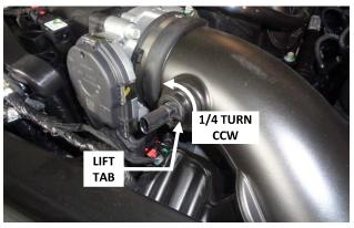
Remove the air temp sensor by lifting the locking tab and turning the sensor a quarter-turn counterclockwise while pulling straight out. Store the sensor in a safe location until reinstallation.
