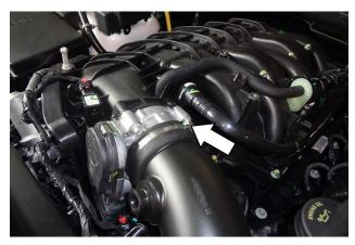
7. Loosen the screw clamp that secures the air inlet duct to the throttle body.
