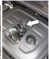
On the engine appearance cover, lift the access panel and remove. Then remove the screw and appearance cover.
