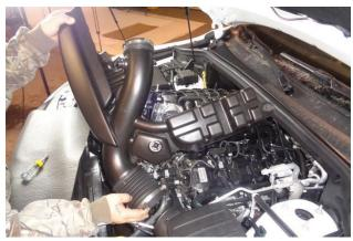
9. Separate the duct from the throttle body and the airbox, then remove it from the vehicle.
