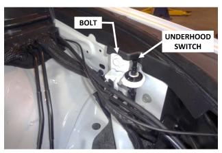
13. Remove the bolt located just behind the hood alarm switch and retain it for use at **Step 21**.
