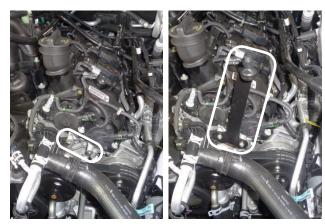
23. Locate the 2 screw holes on the engine as shown, and attach the bracket using M6 screws (8), lock washers (7) and flat washers (6).
