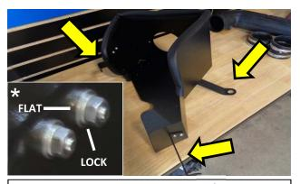
10. First, attach the 3 metal brackets  $\implies$  to the FM heat-shield using the supplied ¼" bolts/nuts and corresponding flat/lock washers installed under the nut-side as shown\*. Tighten all fasteners securely.
