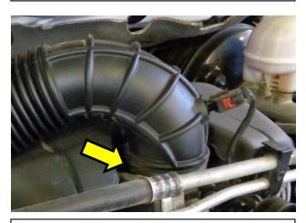
3. Loosen the hose clamp retaining the factory intake tube to the throttle body and remove the entire stock air-box/intake tube assembly from the vehicle by lifting straight up and out. Place the assembly on a flat stable surface for further steps.
