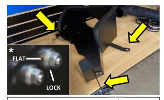
10. First, attach the 3 metal brackets  $\implies$  to the FM heat-shield using the supplied  $\frac{1}{4}$ " bolts/nuts and corresponding flat/lock washers installed under the nut-side as shown\*. Tighten all fasteners securely.
