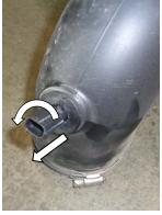
4. With the stock air intake assembly lying on a flat surface, remove the stock air temperature sensor from the intake tube by twisting counter-clockwise and gently pulling outward simultaneously. Next, remove the O-ring from the sensor body and lube the area with a sensor-safe grease. Retain in a safe place.
