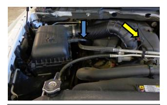
2. Disconnect the air-temperature sensor plug on the intake tube by depressing the rocking tab and gently pulling away. Next, disconnect the crankcase breather hose from the stock air- box. NOTE: We highly recommend that customers retain their factory air intake system.
