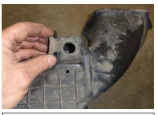
5. Turn the stock air intake assembly over and remove one of the rubber grommets from the base and retain for use on the FM Cold Air Intake System.
