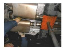
3) Place a supplied 2 ½" clamp onto the inlet of each #842546-Z muffler. Then fully slide the mufflers onto the back of the Scavenger pipe assembly and support with stands. Level the mufflers and tighten the clamps enough to hold, but still allow for adjustment.
