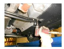
2) Using a 13mm socket, unbolt the two body braces in the center of the vehicle and set aside. The braces will be re-installed after completing step 2 of the installation instructions below.
