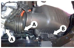
6. Loosen the hose clamps (A) at each end of the air duct, and separate the duct from the airbox.
