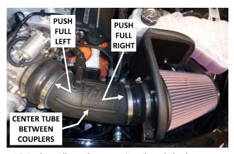
18. Push small coupler up against throttle body stops, and tighten throttle body clamp. Push large coupler up against heat shield, and tighten heat shield clamp. Then center the intake tube between the couplers, and tighten the tube clamps. Install air filter (1) with clamp (2).
