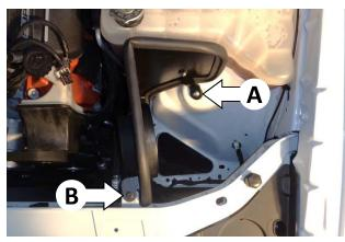
14. Place assembled heat shield in the vehicle. If required, adjust alignment of brackets and retighten their fasteners. Tighten %-16 screw in rubber well nut (A), and secure front bracket (B) with stock screw removed at Step 6.
