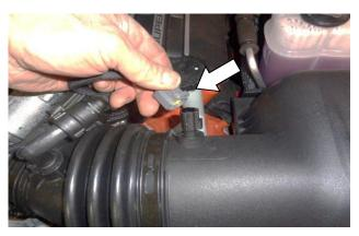
4. Disconnect the plug from the inlet air temperature sensor by depressing the locking tab and pulling the plug straight off.
