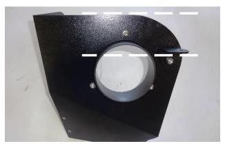
10. Attach bracket (12) to heat shield using ¼-20 screw (9) (against the heat shield), and flat washer (6), lock washer (7), and nut (8) (against the bracket). NOTE: Align bracket so tab is approximately parallel to top edge of heat shield, as shown.
