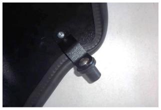
13. Attach rubber well nut (4) to bracket with 3/8-16 screw (11), hand tight only.
