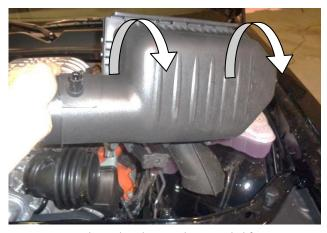
7. Remove the airbox by simultaneously lifting it up and rolling it forward. Then, remove the air duct from the throttle body.
