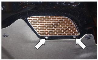
19. If the vehicle is to be driven in wet weather, use of the intake block-off plate (23) is recommended, to protect the air filter from exposure to excess water. Remove the two screws that secure the factory vent grille.
