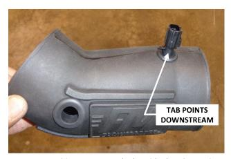
15. Insert rubber grommets (19) and (20) in the intake tube (18). Carefully press the air temp sensor into the small grommet, ensuring that the tab points downstream. (NOTE: Moistening the grommet with soapy water will ease insertion.)
