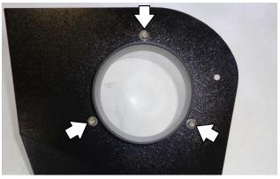
9. Assemble air filter adapter (3) to heat shield (10) using M6 screws (15), lock washers (14) and flat washers (13).
