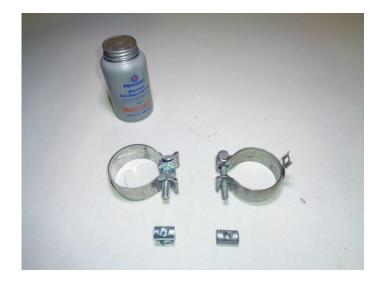
5. Place (x2 ea.) rubber hangers (10) and front frame hangers (6) onto resonator hangers. Use (x2) clamps (7) to connect right (1) and left (2) inlet pipes to scavenger assembly (3). Connect assembly to flanges and fasten front frame hangers to vehicle (logo facing down).
