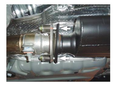
Place clamp (7) onto left muffler assembly (4) then connect it to left side scavenger outlet. Repeat with right muffler assembly (5) on right side scavenger outlet. Tighten clamps enough to allow for adjustment.
