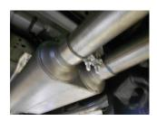
8) Install a provided  $2\frac{1}{2}$ " clamp onto the right muffler outlet. Place the right side tailpipe **#86195S** into position over the axle and slip into the right side muffler outlet, while at the same time, connecting the hangers at the front and rear of the pipe to the rubber mounts on the vehicle. Tighten the clamp enough to hold, but still allow for adjustment.
