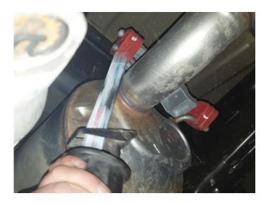
4. Remove grounding wire from hanger and bolts (x2) securing muffler flange. Remove muffler section from vehicle and disassemble flange gasket. Retain gasket for later use.
