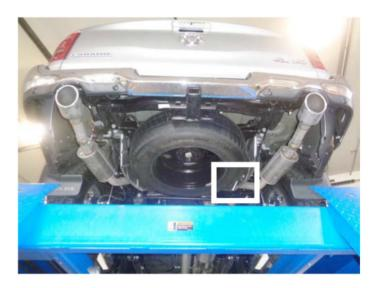
Remove factory tailpipe from vehicle by cutting it near muffler outlet and dismounting wire hangers from factory mounts.
