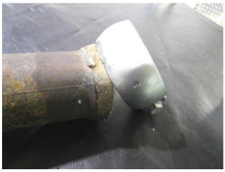
3) Place a factory clamp onto one of the new Flowmaster tips and put up into position behind the resonator on the right tailpipe. Tighten the clamp enough to hold the tip in place and adjust to the desired position. Tighten the clamp securely. Repeat this step on the left side of the vehicle.
