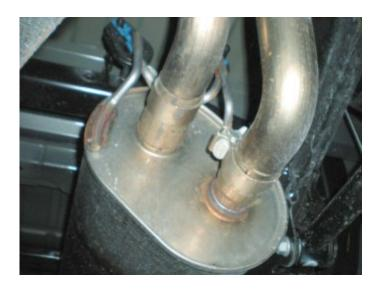
4. Loosen clamp on muffler inlet, then remove hangers (x2) at muffler rear from isolators. Slide muffler rearward to disconnect it from inlet pipe then lower and set it aside.
