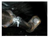
4) Place the provided 3" clamp onto the inlet of muffler **#8530582-258**, then slide onto the factory front pipe and connect the two hangers at the back of the muffler to the rubber mounts on the vehicle. Be sure to line up the notch on the muffler inlet with the tab on the pipe.
