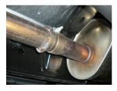
2) Support the muffler with a stand and loosen the clamp on the muffler inlet pipe, then remove the two hangers at the rear of the muffler from the rubber mounts on the vehicle. Slide the muffler to the rear and disconnect from the inlet pipe. Lower and set the muffler aside.
