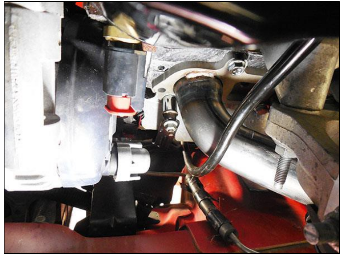
Figure 2 – Dipstick tube mounting bracket spacer w/ OEM bolt
