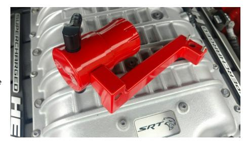
**Step One:** Remove the Supercharged Hemi coil cover on the passenger's side of the engine. It just pulls off with a light pressure.
