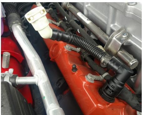
fitting that you need to pull out about a millimeter, at which point it will slide off of the
