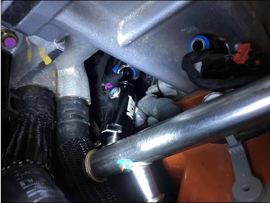
Figure 16 – Fuel Tap Connection
