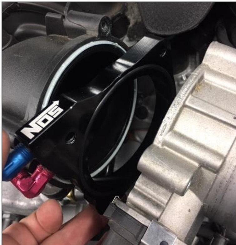
Figure 6 – Nitrous Plate Installation
