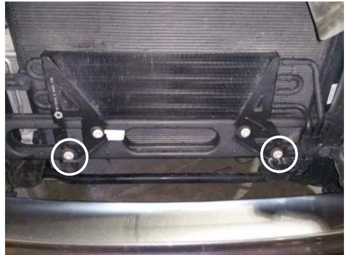
Cooler Bolts Removed
