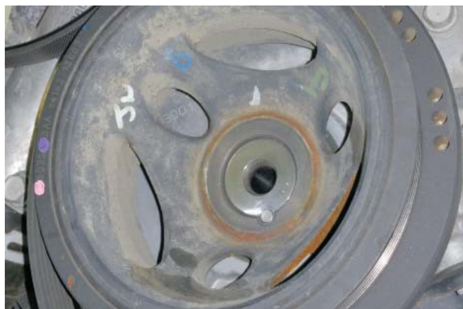
Crank Pulley Pinned to Crankshaft
