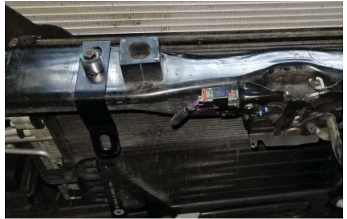
Upper IC Brackets Installed
