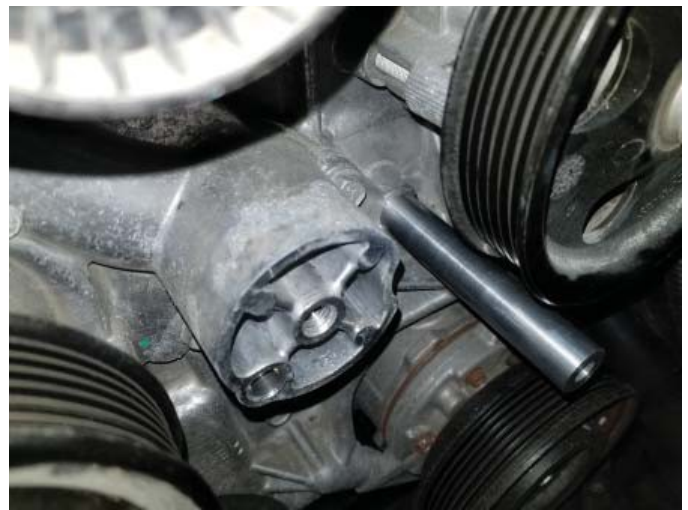
M8 Threaded Spacer Installed
