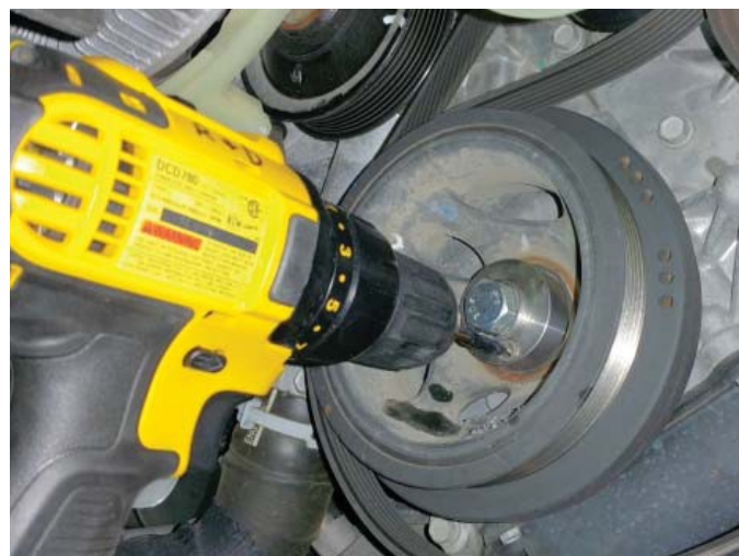
Drill Jig Installed
