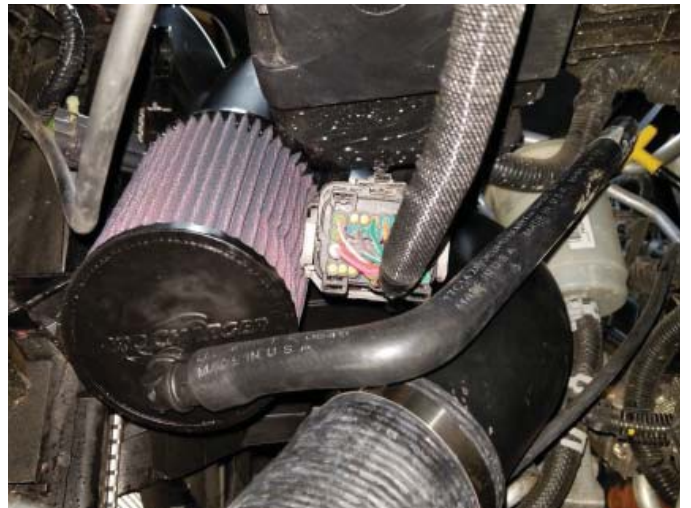
PCV Line Installed
