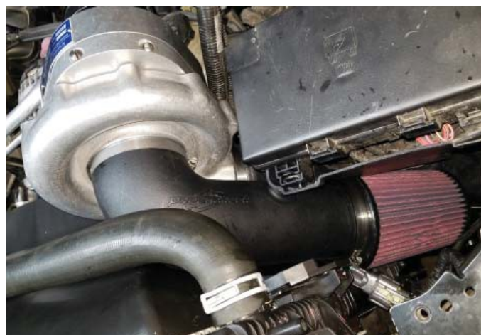
Air Inlet Installed
