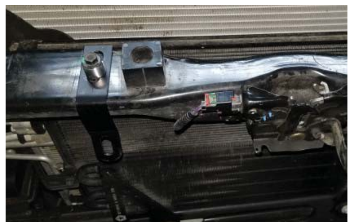
Upper IC Brackets Installed
