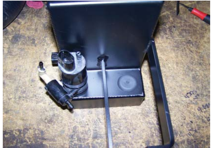
Washer Tank With Pump And Plug
