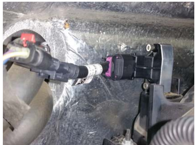
2-Bar MAP Sensor & Adapter Installed
