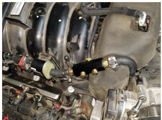
Vacuum Manifold Installed
