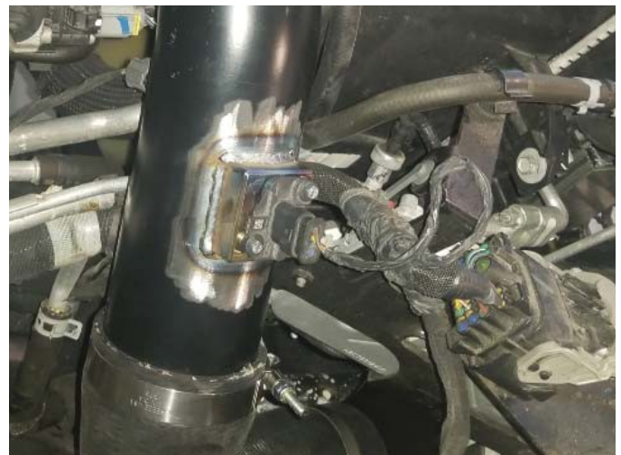
2-Bar MAP Sensor & Adapter Installed
