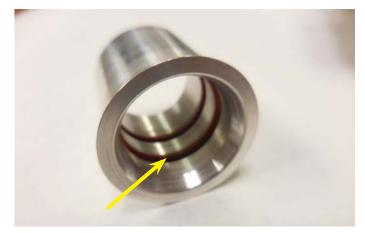
34. Apply a light coat of provided Loctite 680 on the outside of the bushings as shown.
