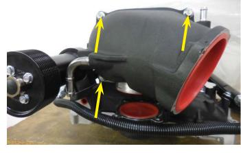
43. Place the provided O-ring in the area shown with the arrow. Secure the factory bypass using the provided four M6x35mm bolts making sure it is centered, and torque them to 108 in-lbs. Place the inlet with the upper rubber coupler onto bypass and secure it back to the supercharger with the four M8-25mm bolts removed in the last step, and torque them to 18 ft-lbs.
