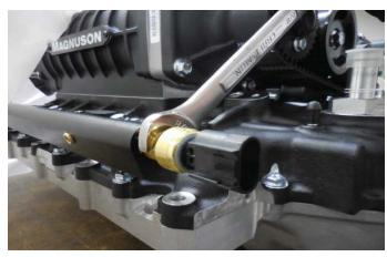
53. Gather the following provided fuel fitting. Apply a light coat of the provided Lubriplate grease to the preinstalled O-ring.
