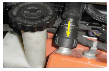
77. Plug in the MAF sensor at the yellow arrow location. Also plug in the throttle control wiring harness at the red arrow location.
