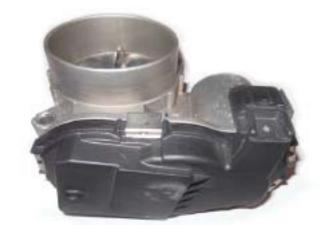
45. Secure the throttle body with the provided M6x45mm bolts. Sandwich the included throttle adapter between the inlet and throttle. Torque the mounting bolts to 108 in-lbs. Verify your torque wrench settings.
