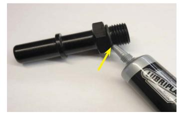
54. Thread the fitting from the last step on the passenger side fuel rail and securely tighten in place with 3/4" wrench. The photo shows the rail removed but this is easier to install while the rail is attached to the blower.
