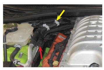
20. Pull out on the red locking clip and press on the release clip to unplug the eight fuel injector connections. Four of these locations are shown with arrows here.
