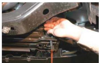
11. Also at this time drain the intercooler fluid. This can be accomplished by removing the spring clamp at the location shown with the arrow and disconnecting the flexible hose from the hard line. Reconnect once the fluid has been drained. Collect this drained fluid in a clean pan and set aside for later re-use.
