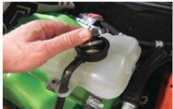
84. Make sure the engine coolant hoses are all connected, and the drain petcock has been closed, strain and re-fill your radiator system with the fluid you drainer earlier.
