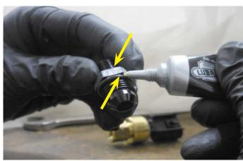
51. Securely tighten the fitting from the last step to the end of the fuel rail shown using a 1/2" wrench.
