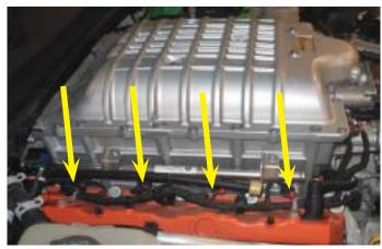
21. Remove the 10 bolts holding the supercharger in place. Five of the left side locations are shown here. The other five are on the opposite side. Have two other people assist you in removing the supercharger. It weighs over 100 pounds so be careful when lifting. An engine lift is recommended if available.
