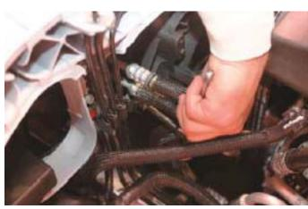
39. Disconnect the fan electrical power connection on the right side of the fan shroud assembly.
