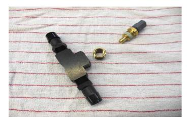
64. Wrap the outside of the threaded reducer with teflon tape, or apply Loctite 567 thread sealant. Install the threaded reducer into the end shown with the arrow.
