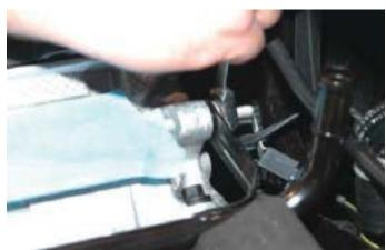
31. Remove the right side heater hard line from the engine. If necessary, you can use a large screwdriver and with the back of the head as a fulcrum, lever the barb free.
