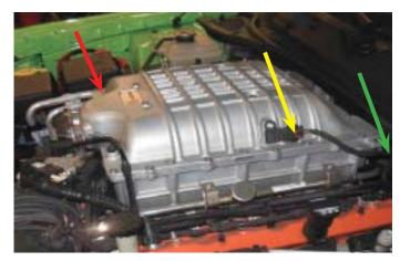
18. Remove the fuel line from the manifold on the right side of the engine. First push the fuel line further onto the fuel manifold barb, then press the locking tabs to release the fuel line, and pull the fuel line free. Use shop towels to capture any residual fuel and dispose of them properly. It's a good idea to cap the fuel rail barb and plug the fuel line to avoid seepage of fuel.
