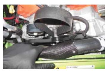
60. Again you will need an engine hoist or a couple of assistants to help you install your Magnuson 2650 supercharger. Carefully lower it into position making sure to line up with the 10 mounting holes. Apply Loctite 242 to the 10 provided M8x60mm supercharger mounting bolts, and install them to the supercharger. Carefully torque these 10 bolts to 18 ft-lbs starting from the inner bolts and working your way to the outer bolts in a criss-cross pattern.
