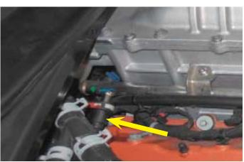
19. Disconnect the upper intercooler hose at the yellow arrow location and the lower at the red arrow location and cap the ends. Be careful of the residual fluid in the lines. Have rags ready for clean up.
