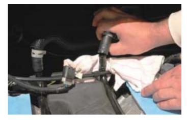
26. Un-clip the grounding connectors on both left and right heads near the heater hard line mounts.
