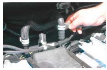
25. Disconnect the two heater hoses from the hard line connection at the rear of the engine by pulling the lines free from the hard line barbs.
