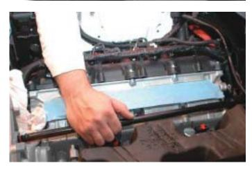
32. Disconnect the wiring mount shown with the arrow and remove it from the electrical harness. Insulate the wire with electrical tape in the area where the mount was removed.
