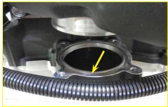
44. Remove the throttle body from the OEM intake manifold assembly using a 10mm wrench on the four mounting bolts.
