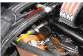
67. Connect the EVAP line at the air inlet (shown with the red arrow), and the brake booster at the yellow arrow location. Also reconnect all the fuel injectors, and the fuel line.
