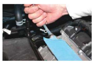
28. There is an additional 10mm hex head bolt holding the left side hard line to the water pump. Remove this bolt using a 10 mm wrench.
