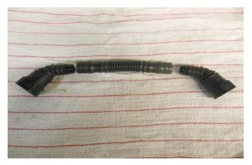
74. Install the two 45° fittings that you removed in the last step to the provided 13" long 5/8" diameter hose.
