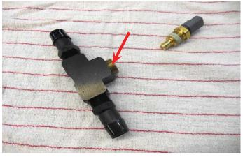
65. Thread the temperature sensor into the reducer that was installed into the last step and securely tighten it.
