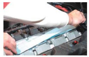
58. Lubricate the cleaned heads with some silicone spray or mild soap solution to facilitate aligning the supercharger on the heads.
