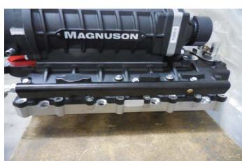
56. Ensure that the plastic slit loom is still attached to the bolt shown before installing the supercharger. This helps prevent the bolt from dragging across the surface of your heads. After the supercharger is aligned with the mounting bolt holes on the heads you can remove this slit loom.
