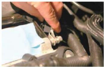
27. Remove the 10mm hex head nut holding the ground sensor and an additional grounding wire to the left side heater hard line mounting bracket/stud at the rear of the head.
