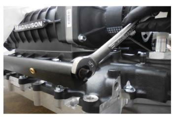
52. Securely install the provided temperature sensor shown at the end of the fitting from the last step using a 5/8" wrench.
