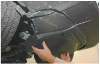
9. The rear splash shield is now dangling. Remove the two rear 10mm hex head bolts holding the rear splash shield to the under carriage and pull the rear splash shield out of the vehicle and set aside the well for later re-installation.
