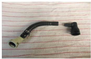
71. Install the 90° fitting from the last step onto the provided half inch hose.
