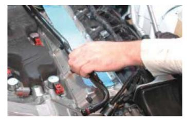
30. Remove the right side hard line mounting bolt/stud on the back of the head using a 10mm wrench.
