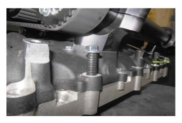
57. Remove the tape or rags from over the ports of the heads. Clean the surfaces using alcohol, acetone, or some other non-petroleum based solvent.
