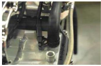
49. Attach the hose that you cut to 3 inches two steps ago to the driver's side intercooler hose barb at the rear of the supercharger lid with one of the provided spring clamps. This hose will also route toward the right side fender, just above the other hose.
