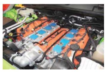
24. Remove the two heater hose clamps from the hard line tubes running forward to the water pump over the valley between the heads of the engine.
