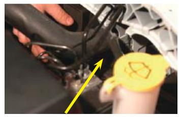
81. Connect the fan control plug to the fan shroud.
