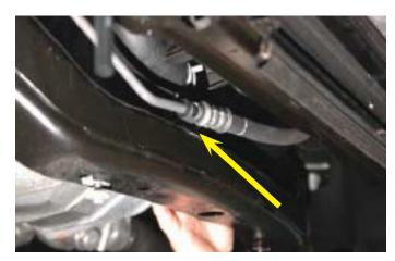
80. Reinstall the two OEM bolts mounting the fan shroud assembly to the framework with a 10mm wrench.
