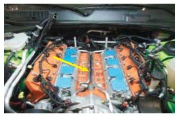
37. Here is another image of the wire from the VVT sensor running up the center of the heater hard lines.
