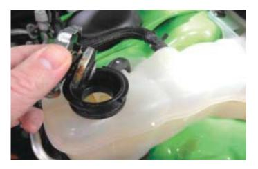
85. Connect the battery negative terminal and key the ignition in the accessory mode to allow the coolant to circulate. **Do Not start the engine at this time**. Recheck the coolant level for the intercooler reservoir and top off as necessary.
