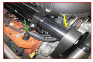
73. Remove the two 45° fittings from the OEM hose shown in the same way you did with the 90° fitting from the previous steps.
