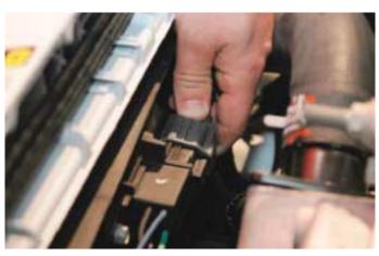
40. Remove the fan assembly from the vehicle by carefully pulling the unit down and out fro reinstallation later. The transmission cooler line mount has a 10mm hex head mounting bolt on the cross frame. Remove the bolt to gain additional clearance on the bottom.
