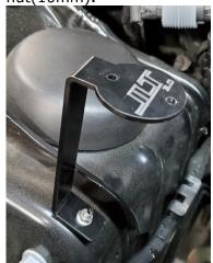
Use the supplied screws and mount the Oil Separator to the JLT bracket. Route hoses to their proper PCV connections. Plug in connections to rubber couplers on vehicle. Reinstall the engine cover.
