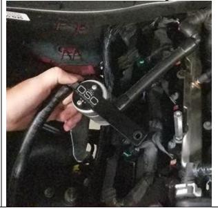
Page 1 of 2 9-21-21 The J&L bracket is going to sandwich between the engine cover and engine cover mounting stud. Reinstall engine cover into rear grommets. Feed bolt into engine cover and J&L Mounting bracket, if you look from the front of the engine, you will be able to see the bolt location to help align it back into the mounting hole. Start bolt by hand and tighten with ratchet.
