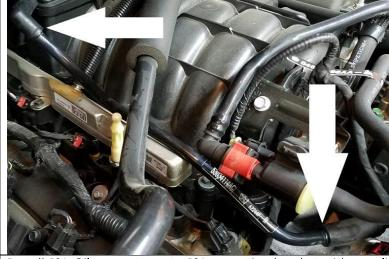
Install J&L Oil separator onto J&L mounting bracket with supplied screws. Logos on bracket and can should 5 line up.
