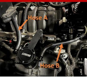
First connect the barbed fittings to the PCV hose ends. Make sure Hose A connects to the side located on top of the engine and Hose B connects to the side on the front of the engine.
