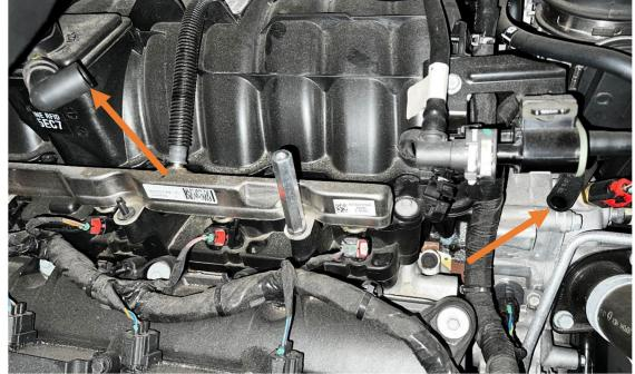
2. Remove factory PCV line from the passenger side of the vehicle in the 2 locations shown.
