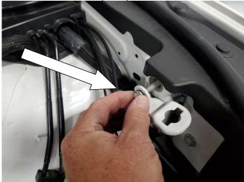
6 Lower heat shield into the area, secure the shield with the supplied push pins in the front scoop FIRST then use the supplied 13mm stainless bolt to secure to the side.
