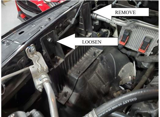
Slide JLT airbox into position with LOWER most locating pin in hole in the bottom of the shield Forward most TAB located BETWEEN fender and airbox mounting tab and rear most tab inside rear mounting hole
