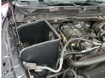
8 Install PCV line into the rubber connection behind oil fill and feed it by the AC lines
