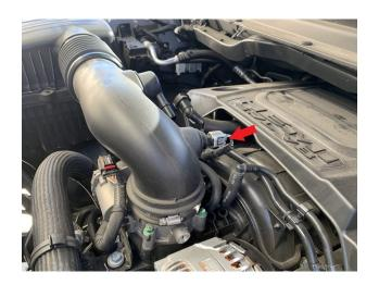
Loosen the hose clamp at the throttle body then pull the intake tube away from the throttle body. Tools Required: Ratchet, 8mm Socket
