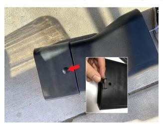
Install the Snorkel Tube and Snorkel Tube Seal (C & D) assembly onto the stock elbow inlet.
