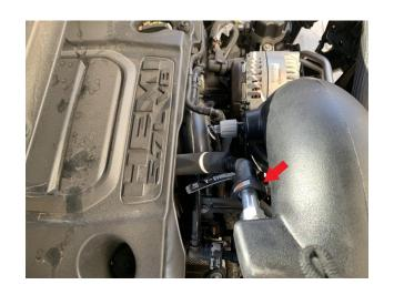
Reconnect the negative terminal on battery. Inspect your installation, make sure the kit is properly positioned and all fasteners are secured. S&B Filter recommends keeping all stock parts in case you would ever need to reinstall the stock intake. Affix the ID label near the intake kit. The installation is now complete. Tools Required: Ratchet, 10mm Socket
