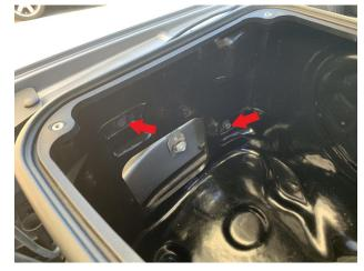
Align the mounting holes on the wheel liner with the Intake Box (A) then tighten with the Bolt (P), Washer (Q) and Lock Nut (R). Fully tighten the two bolts from Step 21. Do not overtighten. Tools Required: (2) Ratchet, (2) 11mm, 13mm Socket
