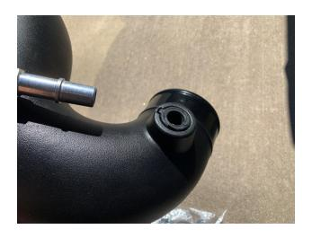
Use a Flat Blade Screwdriver to carefully prop up the locking tab to assist in removing the IAT sensor. Turn the sensor counterclockwise to unlock then pull out. Tools Required: Flat Blade Screwdriver
