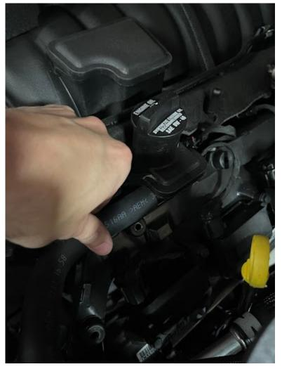
Remove CCV hose from airbox and engine (Some models may have clips securing CCV hose, just use pliers to squeeze them and slide them down the hose)
