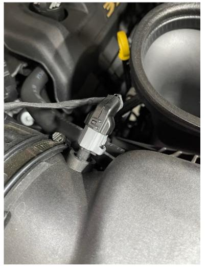
On the stock tube unclip the IAT sensor harness from the stock sensor.
