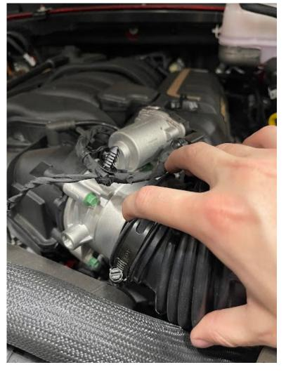
Pull stock tube off throttle body and firmly pull airbox out of the vehicle.
