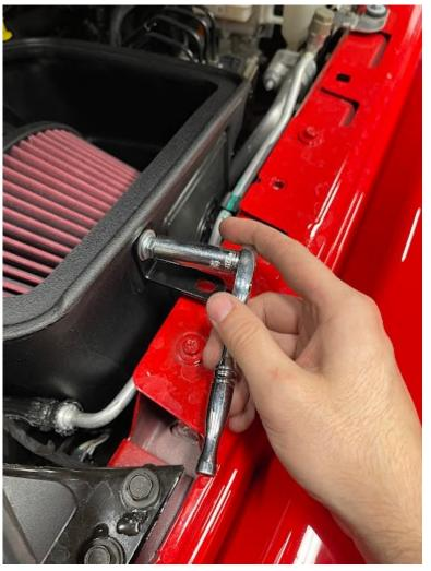
First, install the short side of the angle bracket onto S&B airbox with bolt, washer, and lock nut. Place rubber washer underneath the bracket against the painted side to protect from scratches and reinstall stock bolt into the fender using 10mm socket or wrench.
