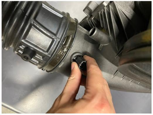
Transfer the IAT sensor from the OEM tube into the S&B tube as shown. The locking tab should rotate over the ramp and lock into position, use the turn arrow for indication.
