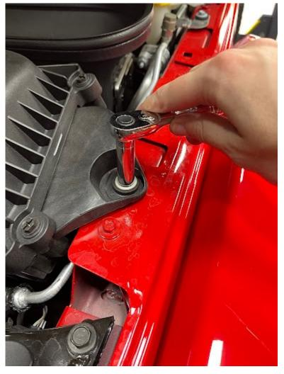
With the engine turned off and cooled down, unscrew the bolt securing the stock airbox on the driver's side with a 10mm socket or wrench. Set the bolt aside it will be reused later to install the S&B airbox.
