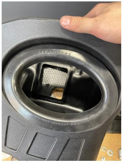
Install silicone tube seal, box plug, and IAT grommet on S&B airbox and tube.
