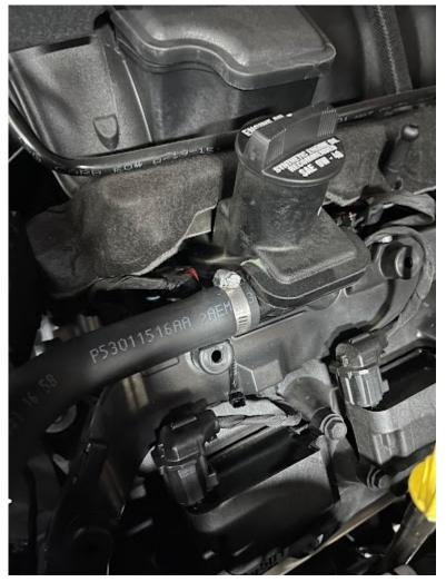
Slide both hose clamps onto CCV hose and tighten using ¼" wrench or flat head screwdriver onto S&B tube and engine.
