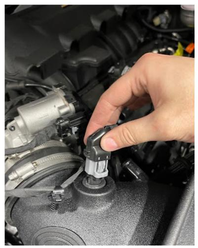
Reconnect IAT wire harness onto sensor, it should clip into place, zip tie harness to reduce slack.
