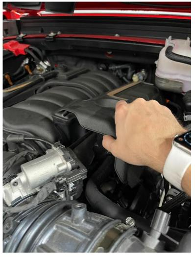
The engine cover is held in place by 2 rubber grommets, firmly lift up on the cover to pop it out of place.
