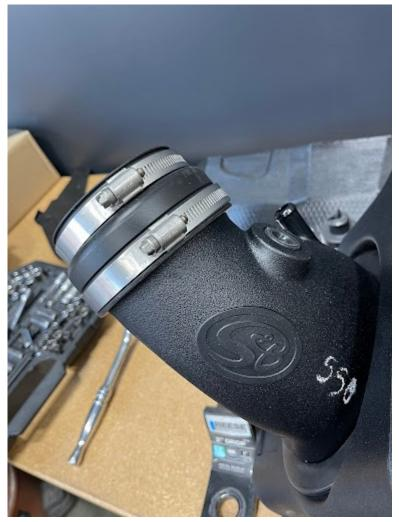
Slide silicone coupler and hose clamps onto S&B tube.
