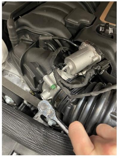
Unscrew the hose clamp on the stock intake tube using a 5/16" wrench or flat head screwdriver.
