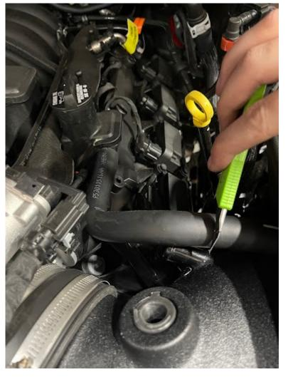
Slide the CCV hose back onto the engine first and then line up the hose with the nipple on the S&B tube. Use a knife or scissors to cut 2-3 inches off the stock CCV hose so that it slides all the way over the nipple on the tube without the hose collapsing in on itself.
