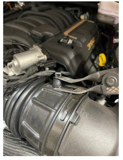
Remove the plastic clips securing the wiring harness using a flat head screwdriver or panel popper.
