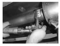
13. Install tail pipe through the rear of the vehicle.
