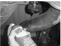
5. Remove the factory tail pipe hanger from rubber isolator.
