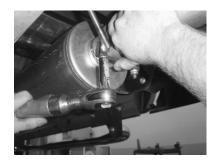
16. Install exhaust clamp loosely over tail pipe. Do not tighten at this point.
