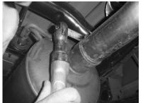
3. Spray lubricant on the exhaust pipe behind the muffler.
