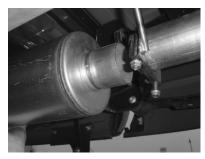
15. Align tail pipe properly and tighten muffler hanger clamp .
