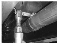
8. Remove muffler hangers from rubber isolators.
