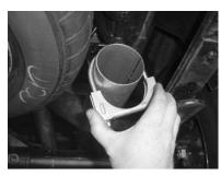
17. Install turnout w/ tip at the end of tail pipe.
