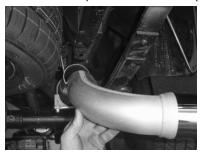
18. Insert turnout w/ tip and hanger into rubber isolator at the rear of the vehicle, near the spare tire.
