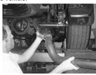
7. Using the 15mm socket and ratchet, loosen the clamp that secures the muffler assembly to the resonator/intermediate pipe.
