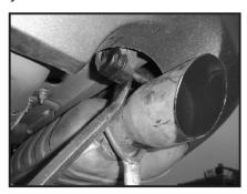
3. Unbolt the driver side rear muffler/tail pipe assembly and remove it.
