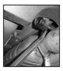
5. Unbolt the driver side rear muffler / tail pipe assembly and remove it.
