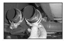
9. Slip the new JBA X-pipe over the end of the catalytic converter.
