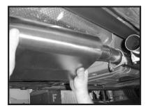
12. Align the mufflers so they are flat then tighten the clamps.
