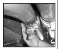
11. Slip the clamps over the end of the X-pipe. Then install the mufflers on to the end of the X-pipe.
