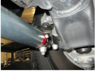
9. Turn the wheels until the rod end of the SWAY-AWAY steering stabilizer is lined up with the other stabilizer mount and reuse the OEM bolt and flange nut.
