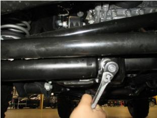
6. <u>Use 18mm and remove the nut from the OEM steering</u> stabilizer mount and remove the bolt on the hub.
