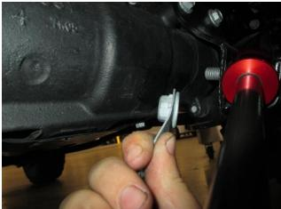
10. Torque down the steering stabilizer bolts to 50 ft-lbs.
